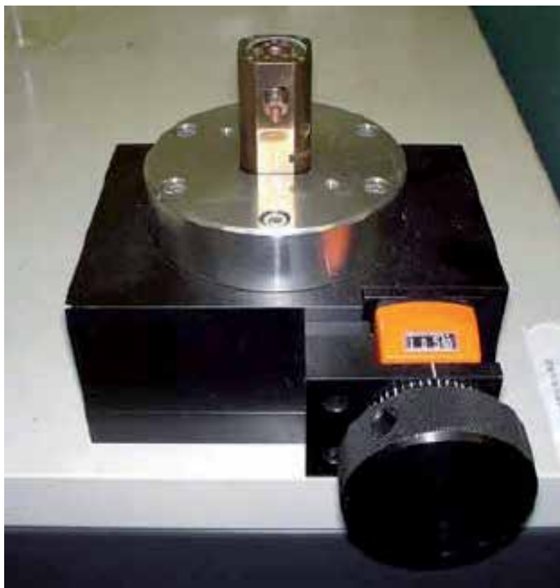
Fig. 3. Schematic picture of diamond anvil cell (DAC).
