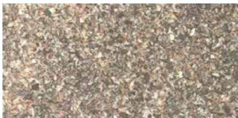
g) 30 % by mass corncob with 70 % lignite mixture
