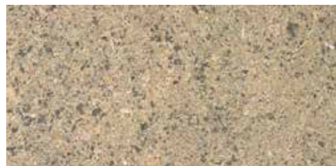
h) 30 % by mass sawdust with 70 % lignite mixture
