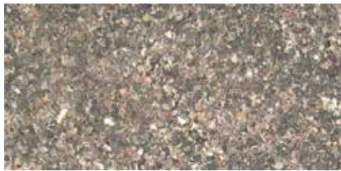
a) 15 % by mass corncob with 85 % pit coal mixture
