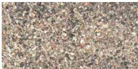
e) 30 % by mass corncob with 70 % pit coal mixture
