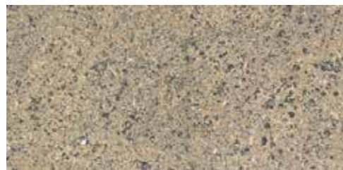
f) 30 % by mass sawdust with 70 % pit coal mixture
