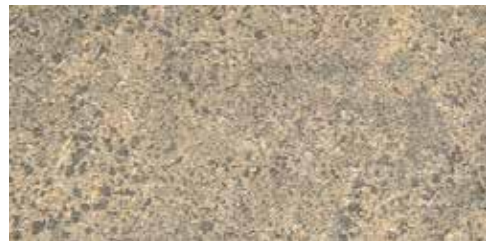
d) 15 % by mass sawdust with 85 % lignite mixture
