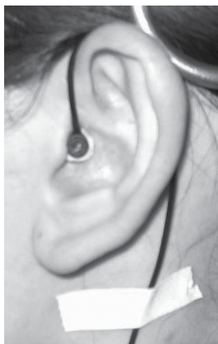
Figure 3. Blocked-ear-canal measurement with miniature microphone
