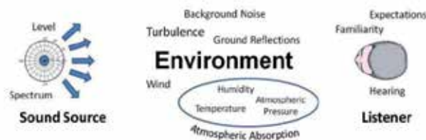
Figure 1. Basic variables that affect auditory distance judgments in an open environment. In a closed environment the additional variables are reflections from space boundaries (echoes and space reverberation) while some environmental variables not present.
