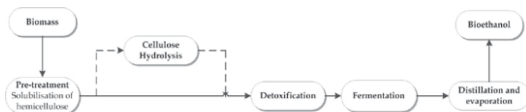
Fig. 6. Schematic steps for production of bioethanol from lignocellulosic biomass
