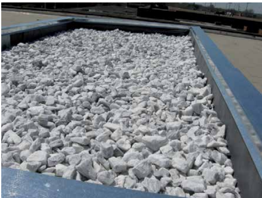
Figure 8. Mini-roof equipped with crushed marble chips.
