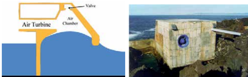
Figure 20. Left side: Schematic of OWC. Right side: Back view of an OWC [37].
