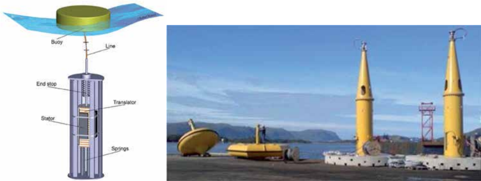
Figure 8. Left side; Taut moored heaving buoy with linear electrical machine PTO [16]. Right side; Component of taut moored WEC, Sweden [22].
