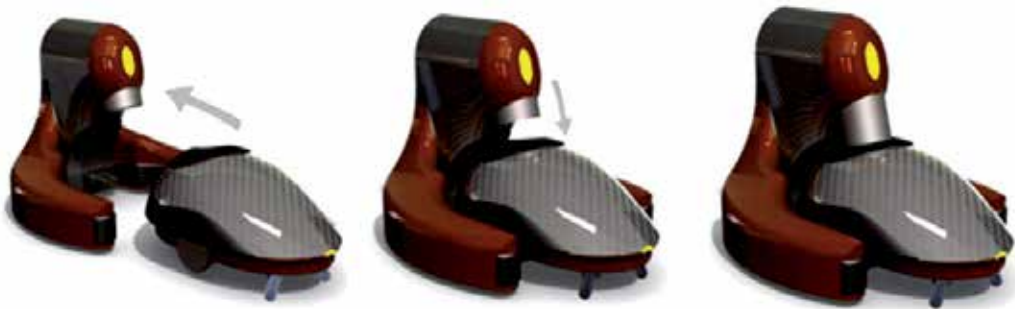
Fig. 6. System for unloading and battery charge of robotic vacuum cleaner.
