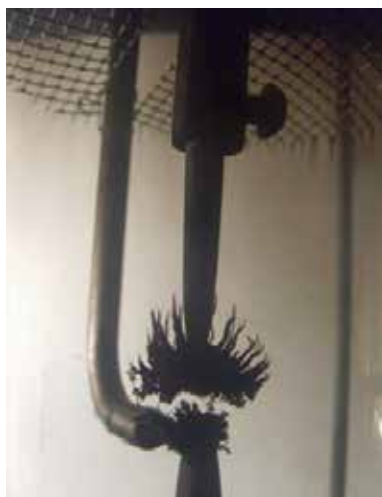
Fig. 5. Carbonaceous depot in both electrodes when ac current is used
