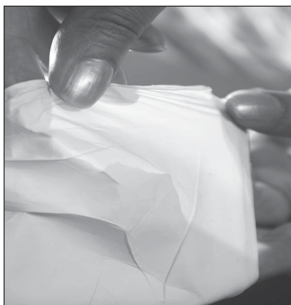
Fig. 2. (a) Basic apparatus for electrospinning, (b) A photo of typical electrospun nanofibre mat.
