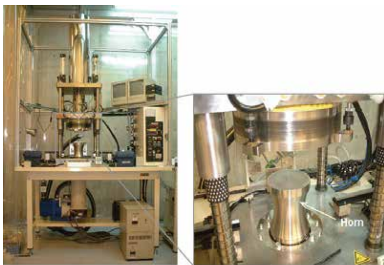
Fig. 2. (a) Photograph of an ultrasonic hot embossing system, and (b) bottom loading stage based on an ultrasonic horn.
