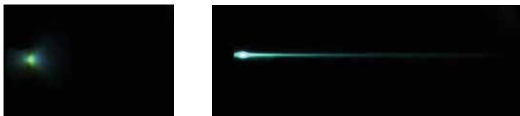
Fig. 7. Plasma images without (left) and with (right) horizontal magnetic field
