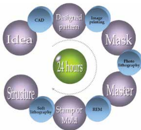
Fig. 2. The rapid prototyping procedure for soft lithography.
