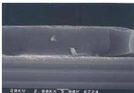
Fig. 15. SEM image of fabricated SU-8 master.
