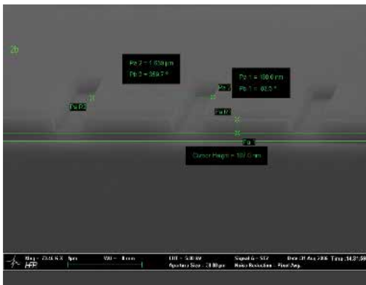
Fig. 13. Close-up of cross sectional SEM picture of imprinted lines and space structure for residual resist measurement (chuck tilted by 80°)
