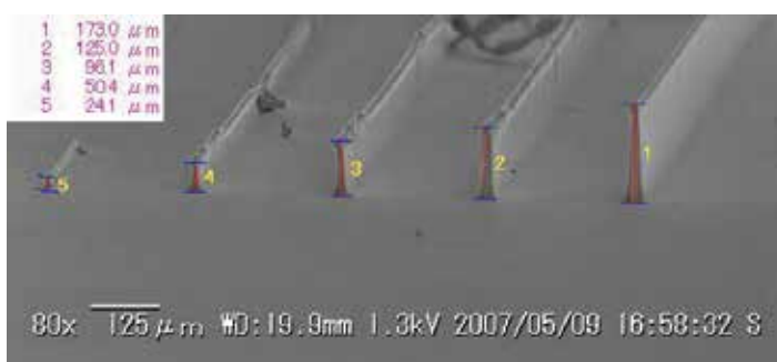
Fig. 3. SEM photograph of different height resist structures for different L&S pattern masks.
