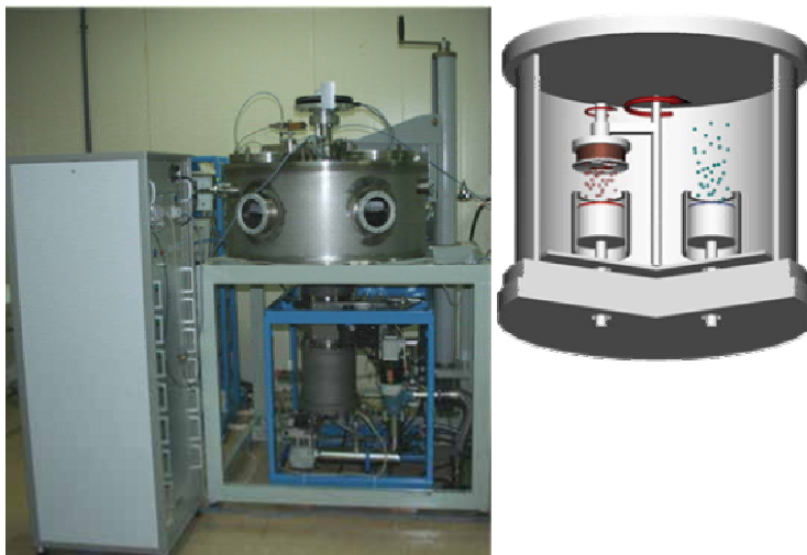
Fig. 24. Photograph of a technological facility and scheme of surface shape correction by means of multilayer film deposition through masks.
