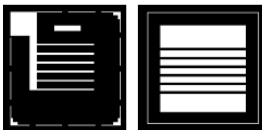
Fig. 10. Masks of device fabrication by MIMIC process.
