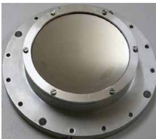
Fig. 33. Photograph of the multilayer spherical mirror for 13.5 nm wavelength in the frame. Diameter of the working aperture is 130 mm.
