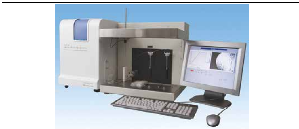
Fig. 7. Photograph of the high throughput, multi-analyte imaging SPR analytical system.
