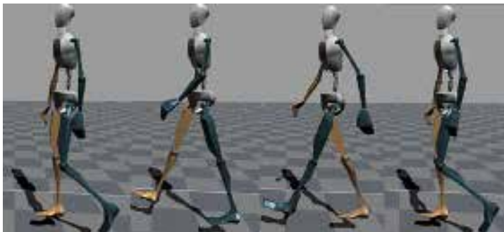
Fig. 2. A sample gait cycle: as received from the wireless inertial motion suit and animated on a 23 DOF avatar within the Moven Studio™ software.
