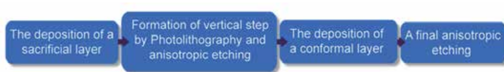
Fig. 1. Step Requirement for fabricating Nanowire using SPL
