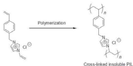
Figure 6. Polymerization of a polymerizable IL having two polymerizable groups to produce a cross-linked insoluble PIL.
