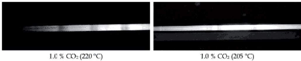
Figure 11. Effect of rheometer temperature on supersaturation of 1 % CO 2 from the CA melt plasticized with 20 wt.-% GTA at constant throughput (11 kg h -1 ) and slit die gap (5 mm).
