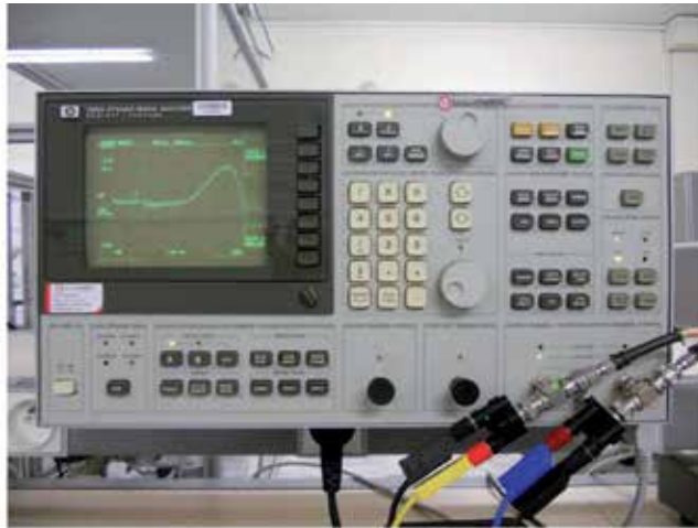
Figure 3. Picture of the double channels Hewlett-Packard HP3561A FFT analyzer.
