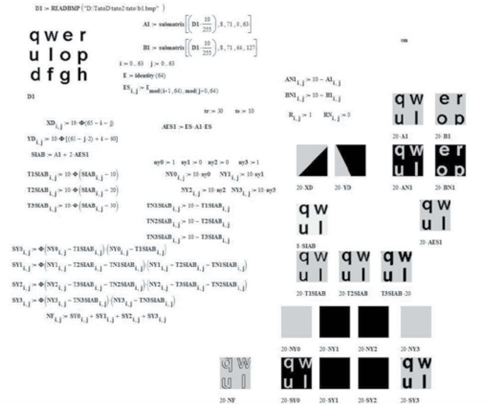
Figure 24. Simulation results of the OPR MFLD-2 with MathCAD for contour extraction
