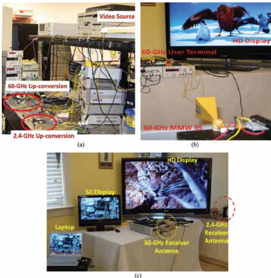
Fig. 39. Transmitter and receiver of the 3-screen, dual-service 2.4-GHz and 60-GHz RoF carrying 270-Mbps SD and 1.485-Gbps HD video content. (a) Transmitter at Centergy lab at 10th Street, (b) 60-GHz Wireless setup at residential lab at 5th Street, and (c) 3-screen receiver at residential lab.
