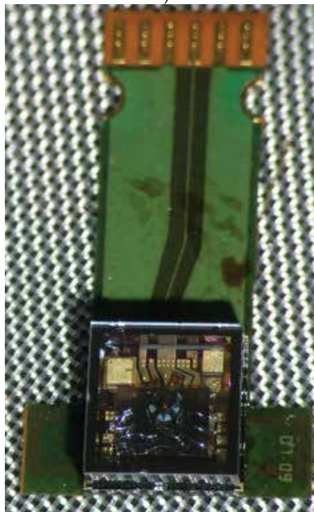
Fig. 13. Assembly of the MEMS device. a) Flowchart of the assembly process. b) Fully assembled system comprising flexprint, MEMS, microlens, electronic components, laser diode and glass lid.
