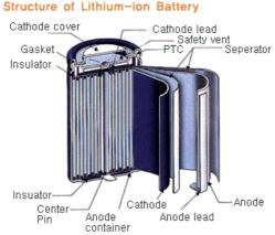
Fig. 10. Structure of Lithium-Ion Battery
