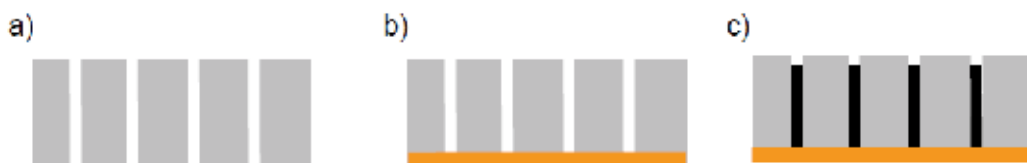
Fig. 7. Schematic of the electrochemical deposition template method: a) nanoporous membrane, b) deposition of a conductive layer on one side of the template, c) growth of the nanowires inside the pores.
