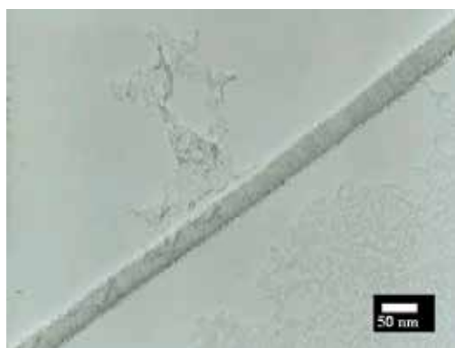
Fig. 3. TEM image of the GaNWs revealing a uniform diameter of \sim 40 nm.
