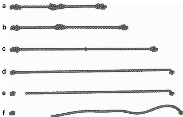
Fig. 2. Three-dimensional views of morphological changes (axial deformation) for CNW (A1). (a) At \varepsilon=0.95 the two parts become a single chain. (b) At \varepsilon=1.42 . (c) At \varepsilon=2.09 the middle part stretches to form a single chain and the stress is the largest (16.65Gpa). (d) At \varepsilon=2.45 the CNW is fully stretched. (e) At \varepsilon=2.457 the chain breaks. (f) After it breaks, the chain recoils.
