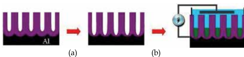
Fig. 6. Fabrication of MNWs via on-substrate AAO/Al template: a) barrier layer thinning, and b) AC electro-deposition.
