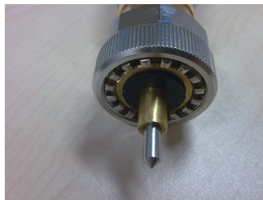
Fig. 7. Test fixture and sample for permittivity from 50MHz to 5GHz
