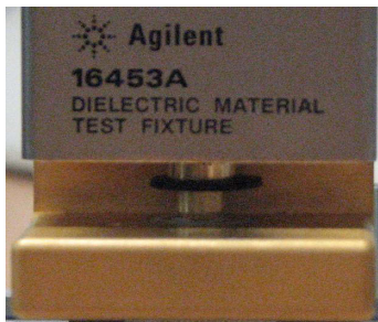
Fig. 6. Test fixture and sample for permittivity from 1MHz to 1GHz
