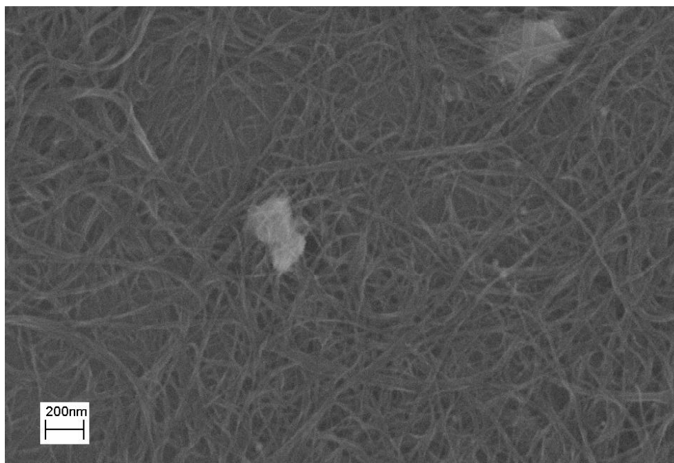
Fig. 1. SEM image of carbon nanotube arrays obtained by LB technique
