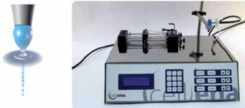
Figure 8. Flow-Focusing technology to make droplets and Cellaena® equipment from Ingeniatics Tecnologías.
