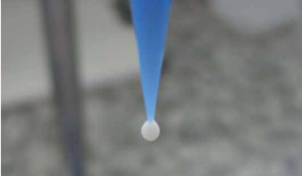
Figure 7. Cell encapsulation in an alginate matrix. Drop generation by gravity using a 160 \mu\text{m} nozzle.
