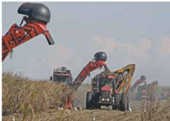
Figure 1. Sugar cane harvester delivering material into a dump trailer for delivery to edge of field (Photo by Sam Cooper, courtesy of Sugar Journal, P.O. Box 19084, New Orleans, LA 70179).
