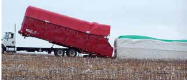
Figure 7. Module hauler picking up module stored at edge of field.
