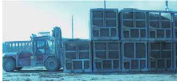
Figure 12. Bins being stacked in at-plant storage at sugar mill in South Florida, USA.
