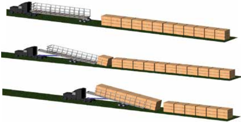
Figure 8. Multi-bale handling unit concept developed for 3x4x8 large rectangular bales by FDC Enterprises-led Consortium (Reprinted with permission [67]).
