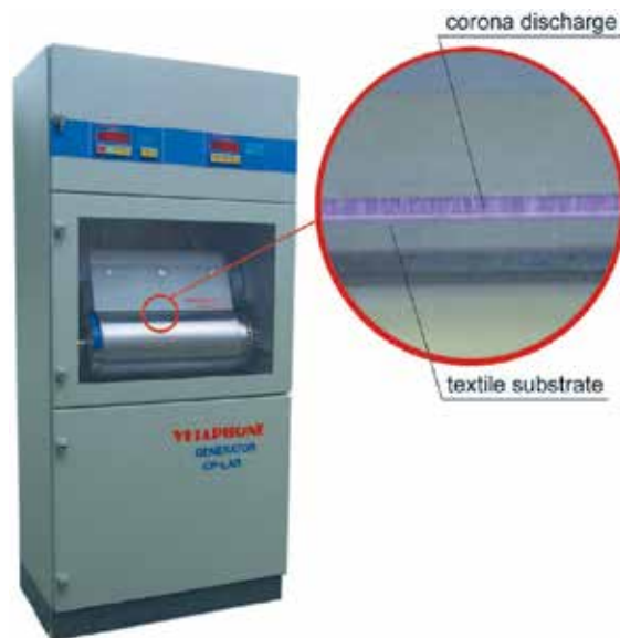
Figure 2. Picture of atmospheric corona plasma reactor and a detail of treating area shown in a red circle
