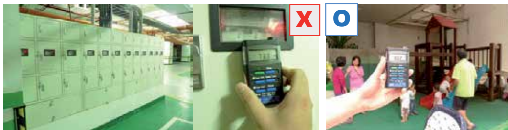
Fig. 19. EMF tests in the electric facility area (left) and the children playground (right)
