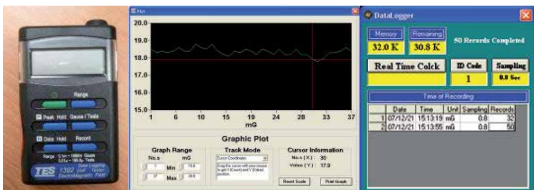
Fig. 6. EMF Tester and operation screen of its software
