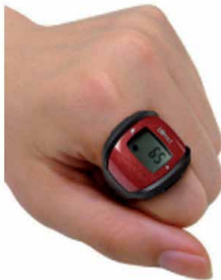
Fig. 2. A commercial ring-type pulse sensor
