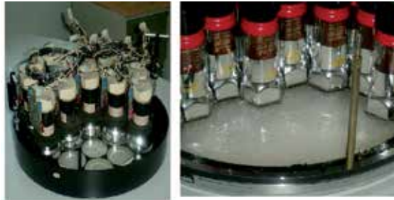
Figure 4. PMTs disposition in a Gamma-camera. Generally a hexagonal shape of PTM is preferred then a circular because it well cover the detection area. Additional very small PMT can also be used between principal PMT for best detection area covering (CEM, Rennes, France).
