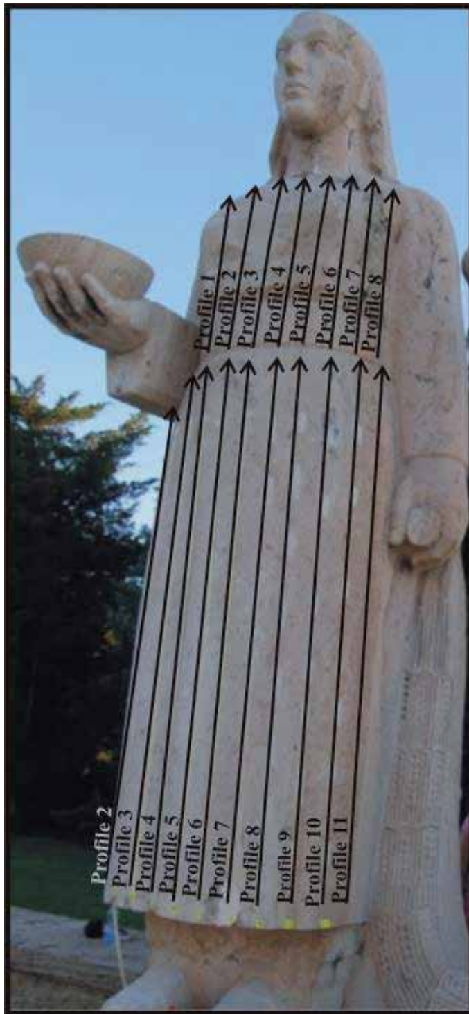
Figure 5. GPR data acquisition scheme of the first female statue.
