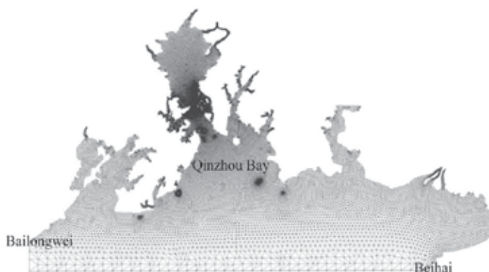
Figure 4. Unstructured grids of Qinzhou Bay.
