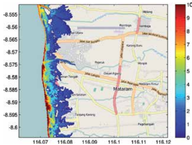
Figure 15. Inundation in Mataram. Flowdepth in the model study based on the Intermap DSM. The bottom roughness is given by a constant Manning value n=0.02 .
