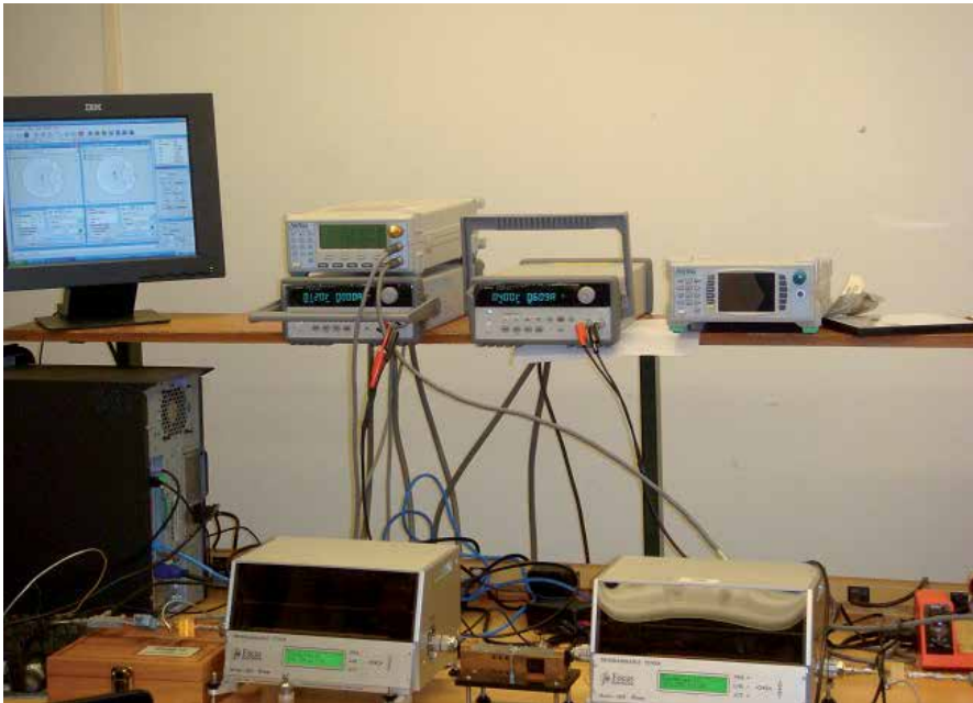
Figure 10. Load-pull bench used to characterize the device
