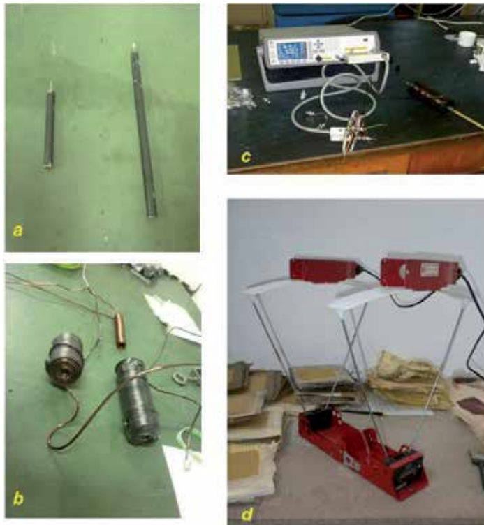
Figure 10. CG set-up pictures: a) short (S) and long (L) iron bullets; b) different copper coils tested; C) inductance static measurements by Agilent LCR Meters; d) ballistic ProChrono chronograph for bullet's speed measurements.
