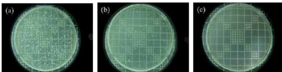
Figure 5. Anti-bacterial performance test of (a) blank, (b) pure PVA and (c) PVA/MWNT-Au nanocomposites nanofibers against the bacteria, Staphylococcus aureus . (PVA solution concentration = 10 wt%, TCD=15 cm, and applied voltage=15 kV)
