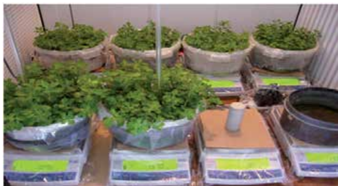
Figure 1. Weighing balance for transpiration measurements
