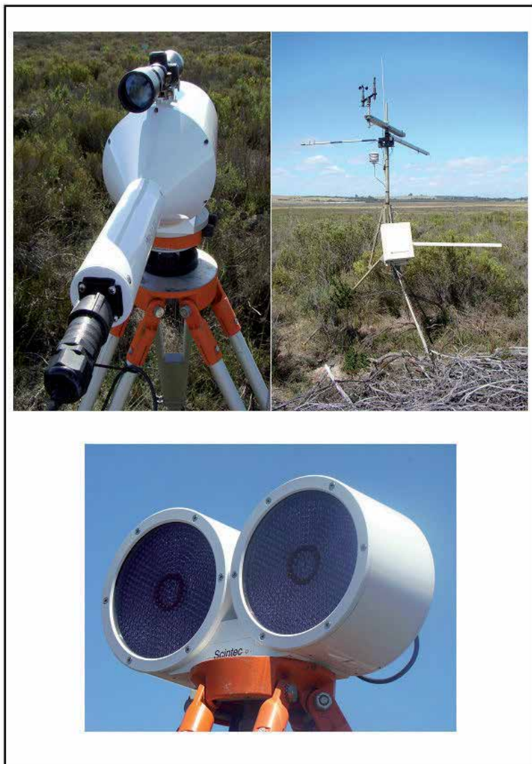
Figure 3. Scintillometer set-up: transmitter (bottom) and receiver (top left) of the scintillometer; and weather station and energy balance system (top right)
