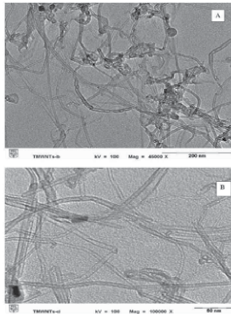
Figure 5. TEM micrograph of MWCNTs after acid treatment with different magnifications (A) 45000 (B) 100000.
