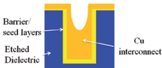
Figure 1. Cross section schematic of interconnect trench or via showing 'super-filling' or 'bottom-up filling' of features through the use of specific plating bath additives for optimum void-free profile evolution in damascene processing [9].
