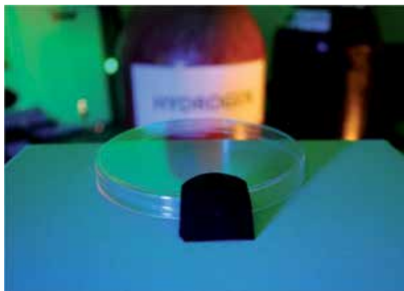
Figure 1. A cross-linked CNT paper with embedded Pd nanoparticles that can be used to construct a hydrogen sensor.
