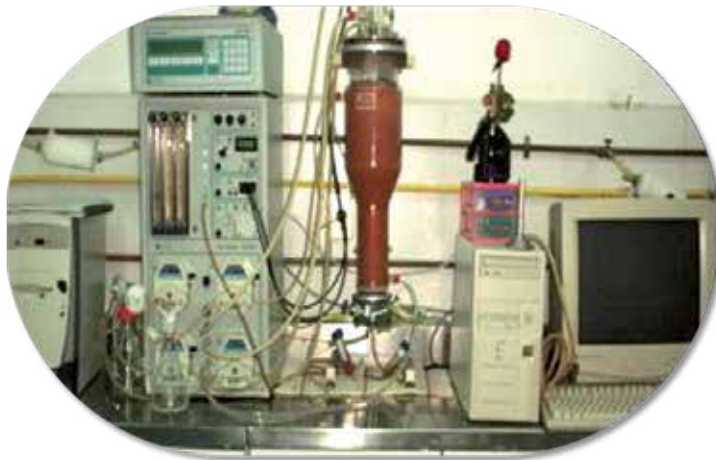
Figure 3. Airlift bioreactor used for the process for Bikaverin production
