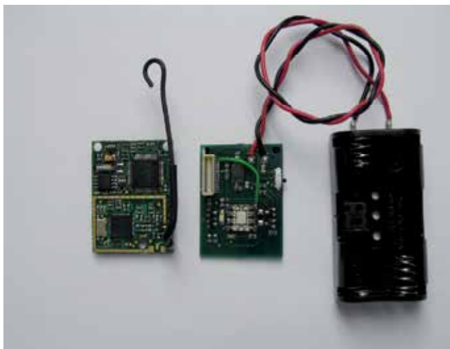
Fig. 6. Construction of PPG body sensor that consisted of a WSN device (left), an PPG front end circuit board (centre) and a battery holder (right).
