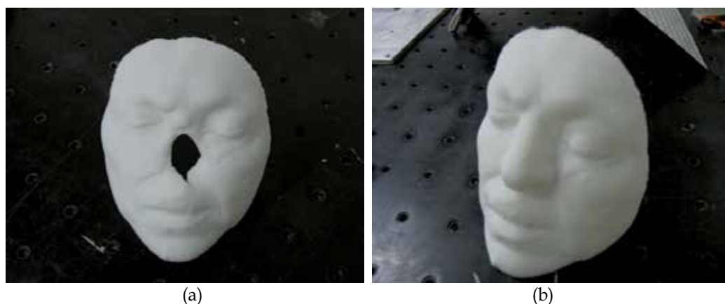
Fig. 4. Physical models obtained by means of rapid prototyping. (a): Model of the original face, internally extruded; (b): Model of the repaired face, externally extruded
