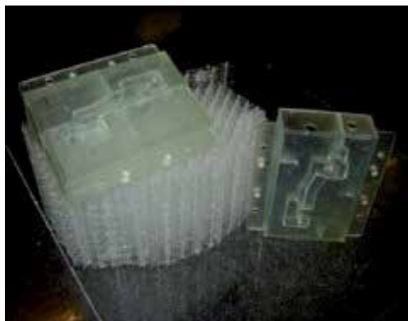
Fig. 21. Fabricated inserts of Peugeot engine gearbox shift fork using stereolithography
