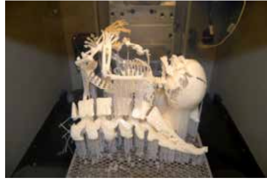
Fig. D. 34 weeks Physical model of fetus built from CT scan through SLA process (3D systems – VIPER Si).
