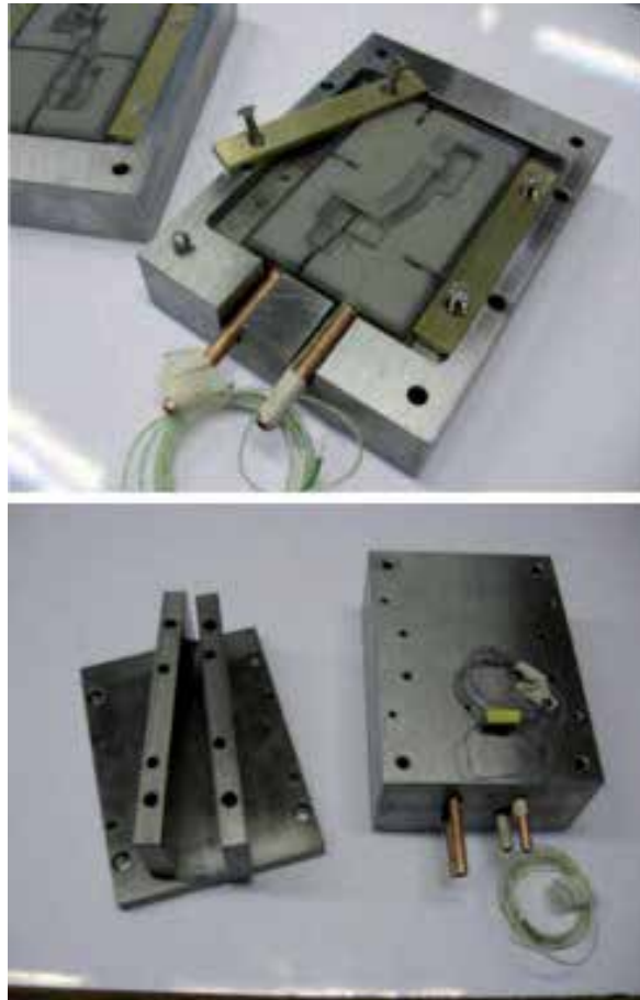
Fig. 14. Tool assembly components and the steel frames
