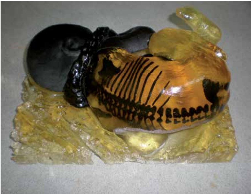
Fig. N. 32 weeks physical model of fetus built in Objet Connex 350 showing the skeleton and the structure of the uterus (transparent).
