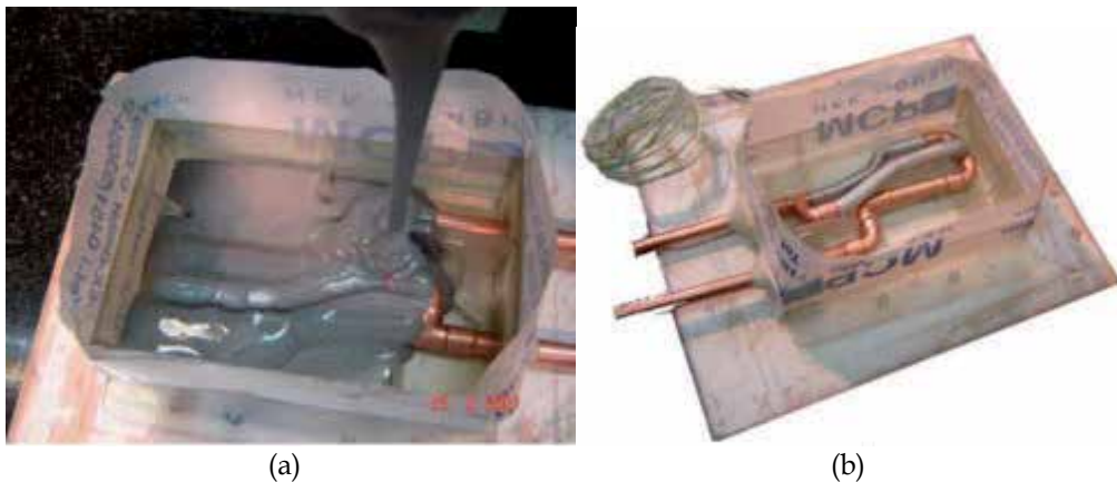
Fig. 23. Back-filling inserts along with copper cooling pipes
