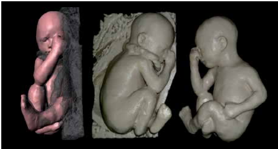
Fig. E. 32 weeks fetus built on Z Corp 510 from MRI files – on the left including the uterus and the umbilical cord and on the right only the body of the fetus.
