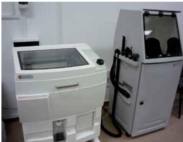
Fig. 6. Z 310 Plus printer and its depowdering station (compressed air system and vacuum suction system) - Transilvania University of Brasov
