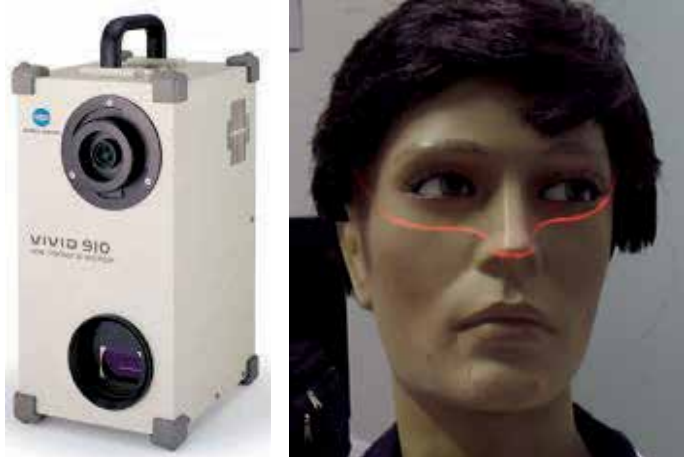
Fig. 1. The optical digitizer Minolta Vivid 910 (left); example of stripe deformation (right)
