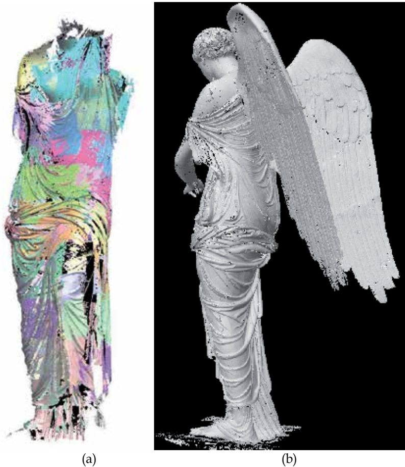
Fig. 22. Acquisition of the whole statue. (a): Aligned high-resolution views; (b): Whole point cloud of the statue
