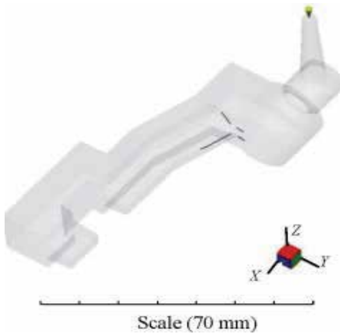
Fig. 17. Wax model weld lines
