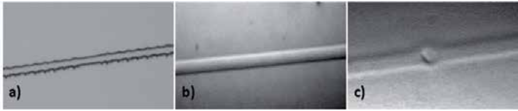
Fig. 16. Waveguides sections written in s-bend. a) Curve defined by short straight lines, b) curve defined by an arc segment, c) transition point between two adjacent line segments.
