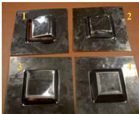
(b) Testing part with different forming angle: 1 – 80°, 2 – 75°, 3 – 68°, 4 – 63°
