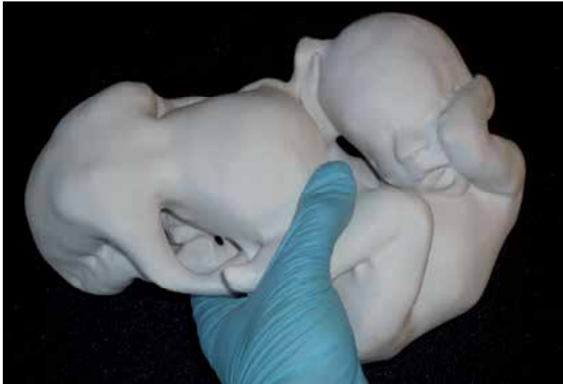
Fig. S. Physical model of 28 weeks twins built on Z-Corp 510 from MRI scan allied to Ultrasonography 3D.
