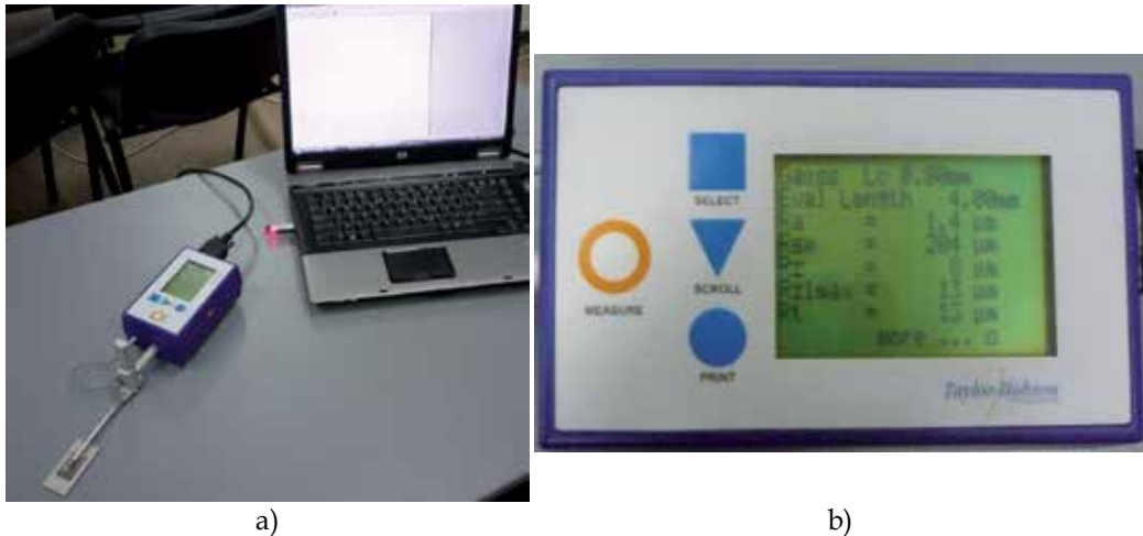
Fig. 32. The parameters calculated by “Surtronic 25”
