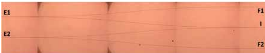
Fig. 37. Coaxial two beam combiner obtained by photographs stitching.
