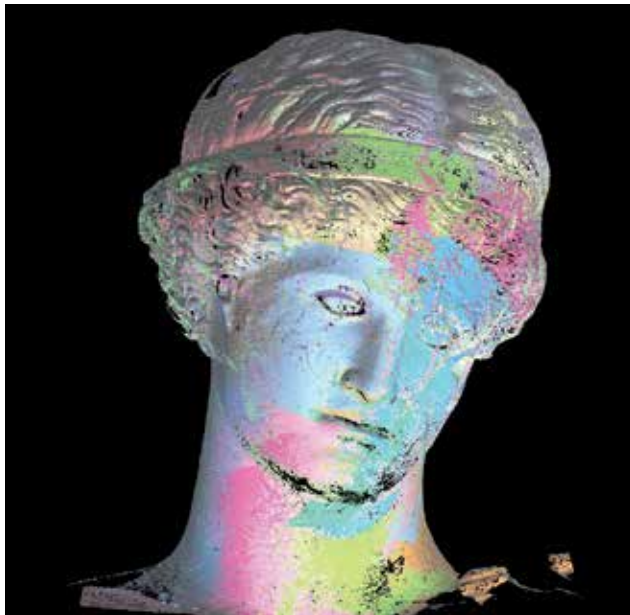
Fig. 19. Multi-view acquisition of the head of the statue (adjacent views are taken with a 40mm overlapping)
