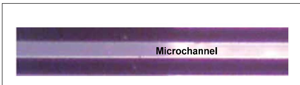
Fig. 1. Color on-line. Photograph (taken under 60 fold magnification) of a wet-etched microfluidic channel on crystalline Si that was used for fabrication of microplasma devices. See text for discussion.
