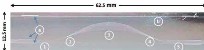
Fig. 32. Arrayed waveguide grating device before the cladding deposition (complete and at scale). a) Marks for waveguides area identification, b) linear waveguides, 1 and 5 input/output waveguides, 2 and 4 free propagating zones and 3 waveguides array.
