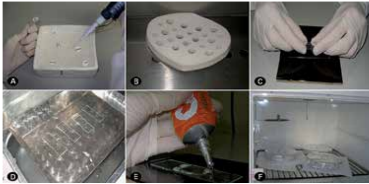
Figure 7. Genomic in situ hybridization. (A) Preparation of the hybridization mixture. (B) Denaturation of the probe at 75 °C. (C) Addition of the hybridization mixture in the chromosome preparation and covering with a glass coverslip. (D) Denaturation of the chromosomes in a metal plate inside a water bath at 73 °C. (E) Sealing the coverslip with rubber glue. (F) In situ hybridization at 37 °C. A, B, C, D and E: Ana R. Oliveira & Ana C. Brasileiro-Vidal; F: Sandra P. Brammer.
