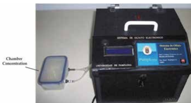
Fig. 6. Chamber of concentration, container for the different samples to be analyzed.
