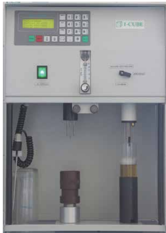
Fig. 4. Foam stability tester type FA by 1-CUBE.
