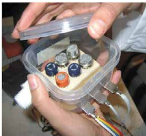
Fig. 3. The chamber of sensors provides hermetic isolation and guarantees reliable measurements.
