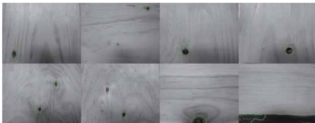
Fig. 8. Segmentation of images acquired with standard lighting visual system (first set).
