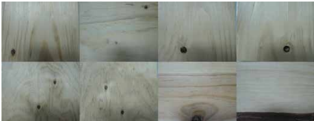
Fig. 1. Defects, knots and splits, on images acquired from a standard lighting visual surface inspection system.
