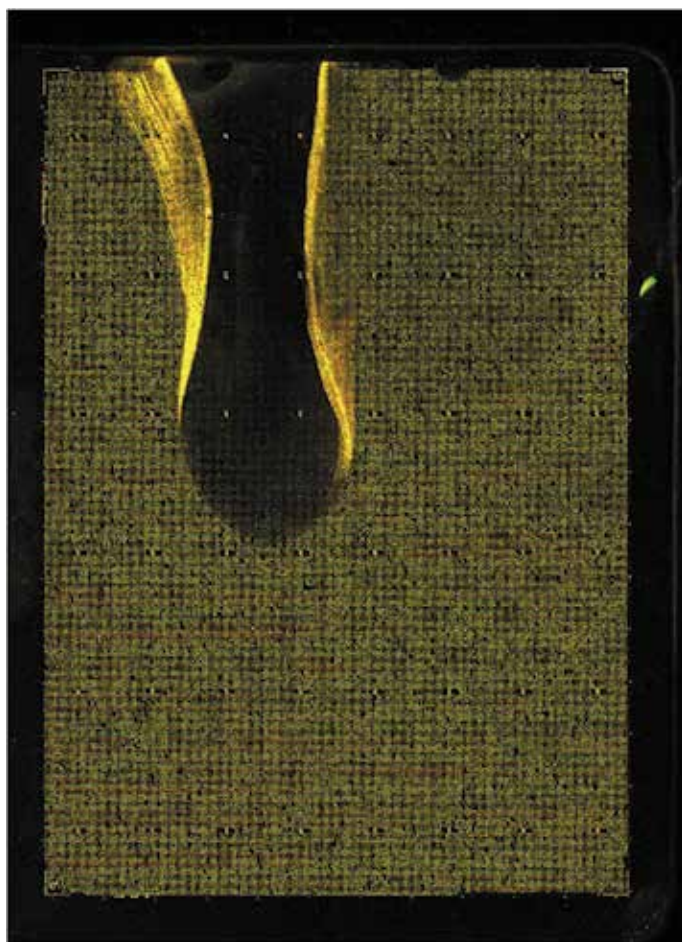
Fig. 2. Microarray after hybridization with an air bubble. The air bubble creates an area of incomplete contact of array product to the hybridization area, which compromises the array.
