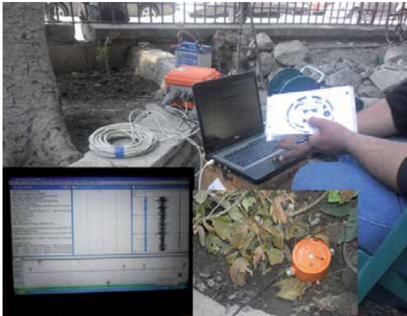
Figure 13. High dynamic range ES-3000 Geometrics mobile station and triaxial geophone used 4 Hz to drive soil response of El-Sakakini Palace.
