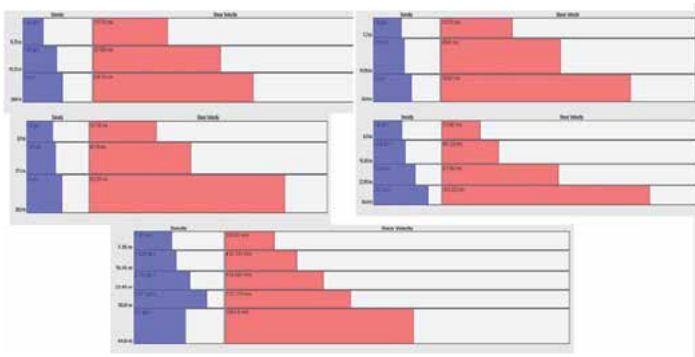
Figure 12. Shear wave velocity model calculated for refraction microtremors profiles ReMi-1 To ReMi-5 (Figure 9).
