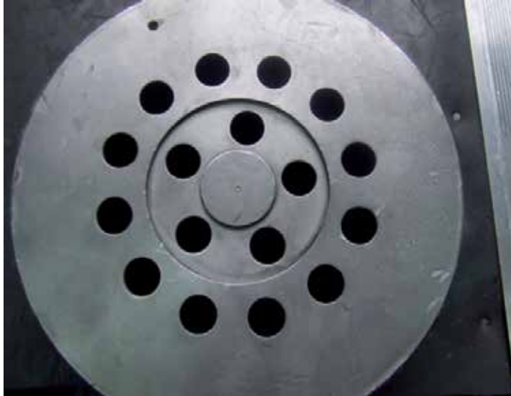
Figure 15. Schematic diagram of 17-hole die with ring-shaped pocket.
