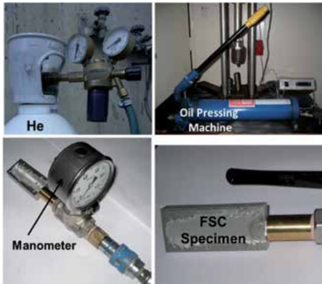
Figure 35. Airtightness and internal hydraulic pressure tests apparatus.
