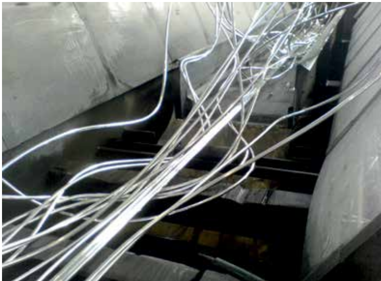
Figure 1. Entangled bars at press run-out, extruded through multi-hole die at non-uniform outflow velocity (Courtesy of Grupa Kęty).
