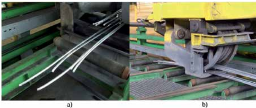
Figure 16. Extrusion of bars through a 17-hole die with ring-shaped pocket, view of bars after exiting the die, b) guiding puller (courtesy of Grupa Kety).
