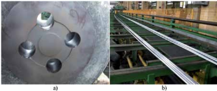
Figure 11. Extrusion tests in industrial conditions through four-hole die, view of ring-shaped pocket die, b) view of extruded bars at press run-out.
