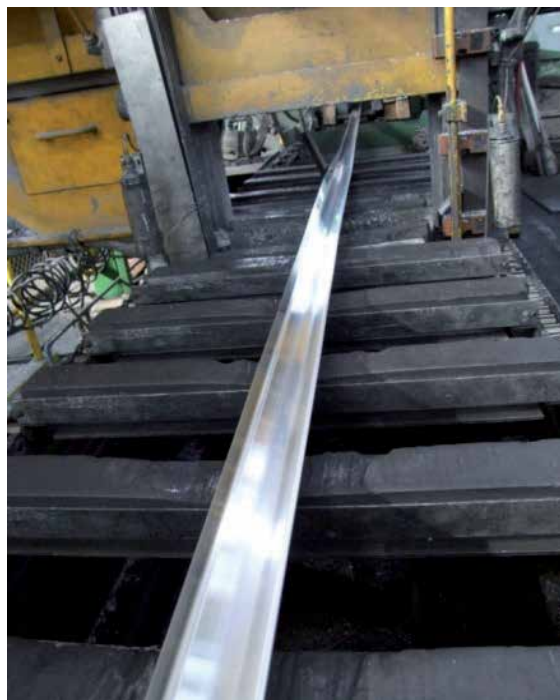
Figure 21. View of 5083 alloy profile at press run-out extruded through pocket die (Courtesy of Grupa Kety).
