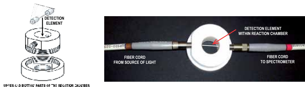
Figure 13. Schematic (a) and manufactured (b) the evanescent wave cuvette of a new design for polymerization on a side surface of the fiber core and recording the hydrogel swelling/de-swelling kinetics. The status of the hydrogel on fiber core can be controlled microscopically in the course of polymerization and swelling/de-swelling. Detection element is a removable part allowing for characterization by the other methods (e.g. atomic force microscopy).
