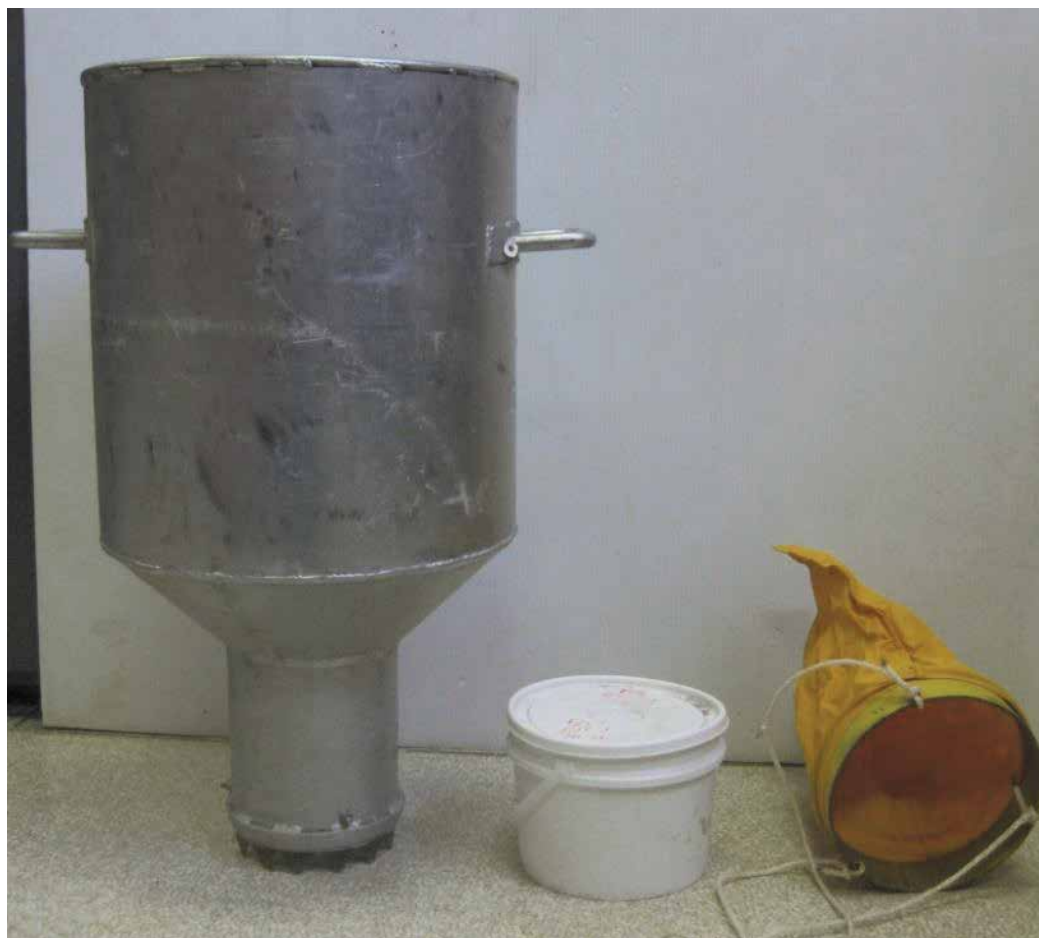
Fig. 1. Laboratory photo of the McNeil corer, gravel bucket, and infiltration bag sampler.
