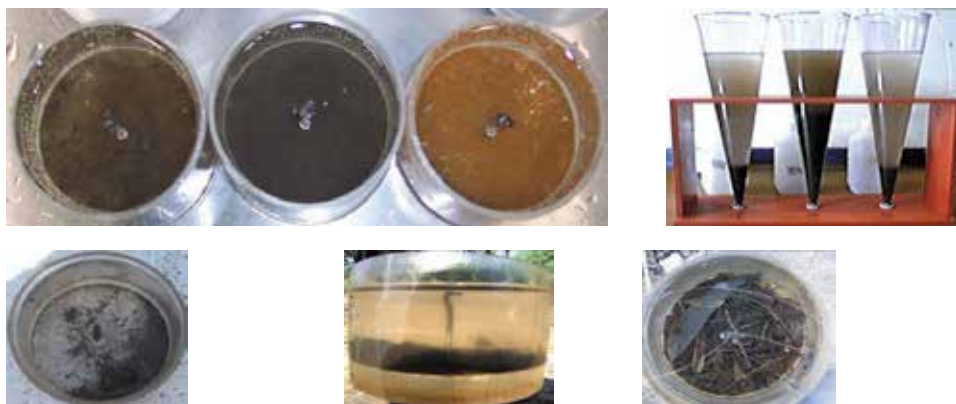
Fig. 10. Example of sediment appearance in the traps and measurement in the Imhoff cones
