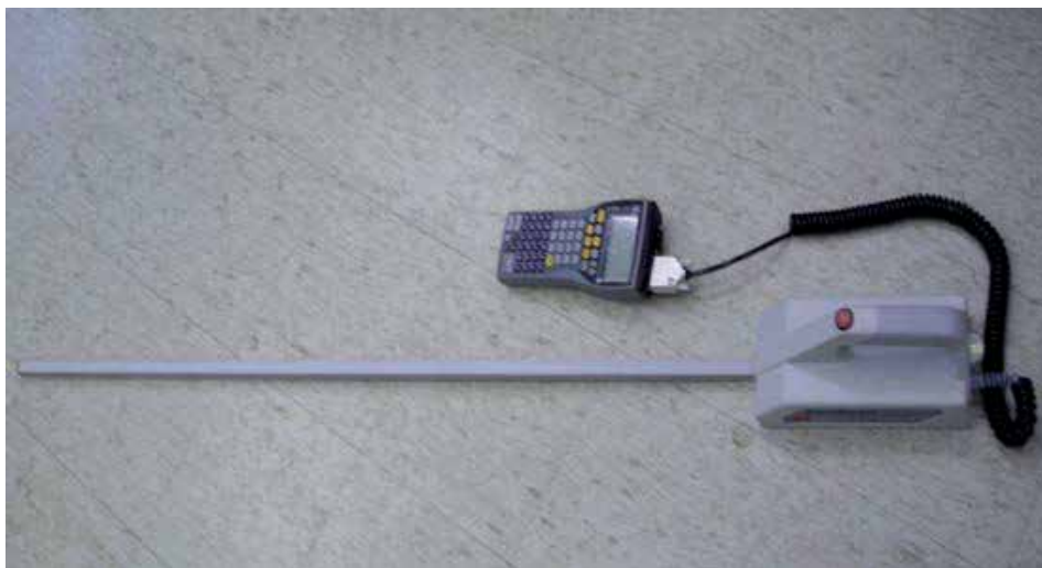
Figure 4. SunScan (Delta-T) canopy analyser for LAI and crop height measurements
