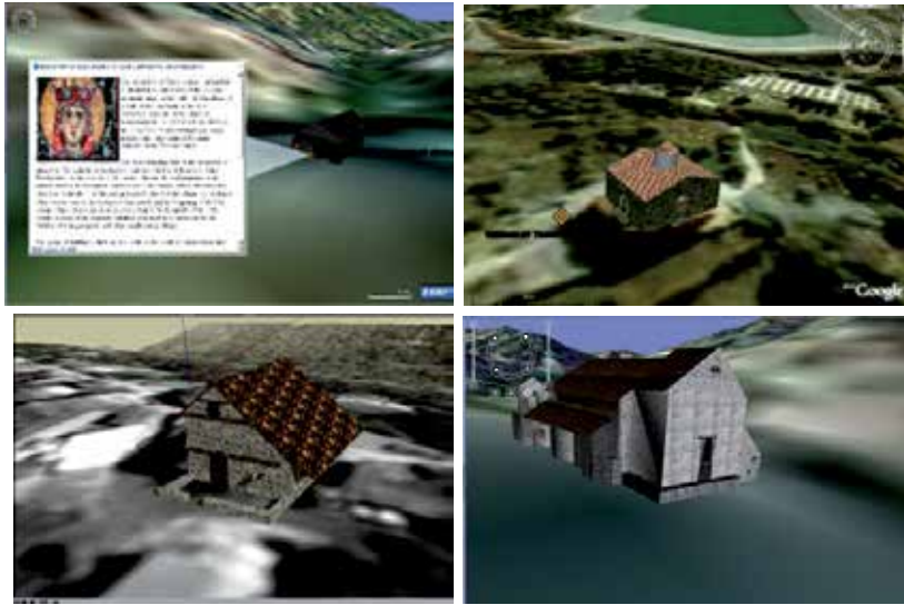
Figure 22. Models for Byzantine and Post Byzantine churches of Cyprus using topometric measurements and GIS tools (Agapiou et al., 2010c).
