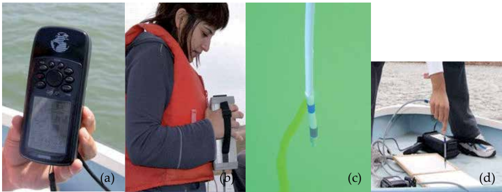
Figure 6. Equipments used during field campaigns (a) Global Position System Garmin GPS72; (b) handheld GER-1500 field spectroradiometer; (c) fibre optic probe & (d) standard Spectralon panel.
