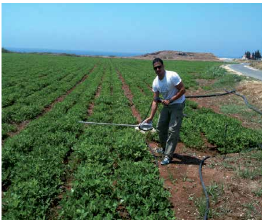
Figure 5. Use of SunScan canopy analyzer for LAI measurements (Papadavid, 2012)
