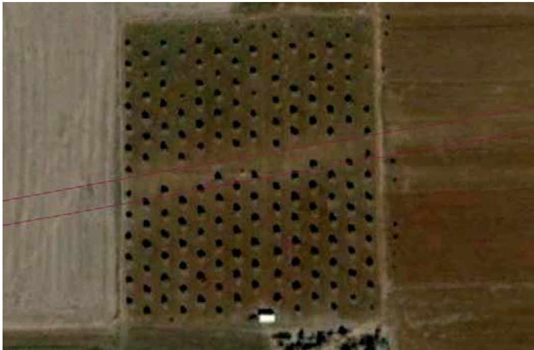
Figure 13. The footprint of the water pipe as a result of the tree pattern.
