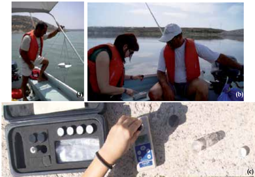
Figure 7. Measuring the turbidity in Asprokremmos Dam using both (a) the Secchi Disk and (b&c) the portable turbidity meter; Palintest Micro950.
