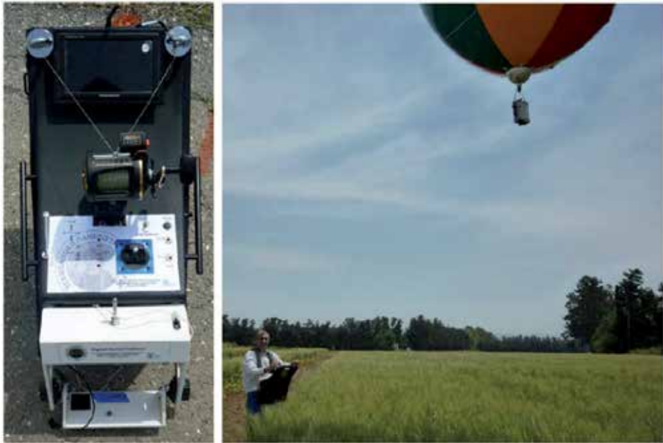
Figure 27. Right- ground control mechanism and aerial platform. Left-Low altitude airborne system including air balloon, spectro-radiometer, and researcher wearing ground control mechanism with harness (Themistocleous et al., 2012b)
