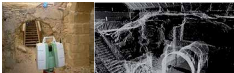
Figure 19. Data collection from the church of Saint Theodore in Idalion village (left). Registration of the point clouds for Saint Theodore in Idalion village. All point clouds are transformed into one coordinate system (right) (Agapiou et al., 2010b).
