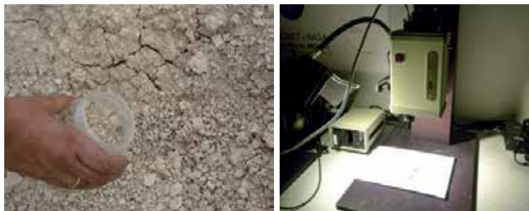
Figure 2. Collection of soil data (left). Spectroradiometric measurements of material samples at the premises of the Remote Sensing and Geomatics Laboratory of CUT (right)
