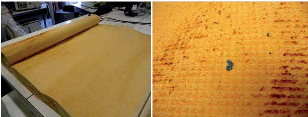
Fig. 8. Iron deposit on RO membrane
