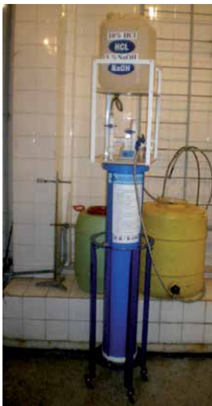
Fig. 13. Photography of a multi process ion-exchange and sorption small water conditioning device (Zvezdov A.,1997; Zvezdov A.,1999; Zvezdov A., et al.2006)
