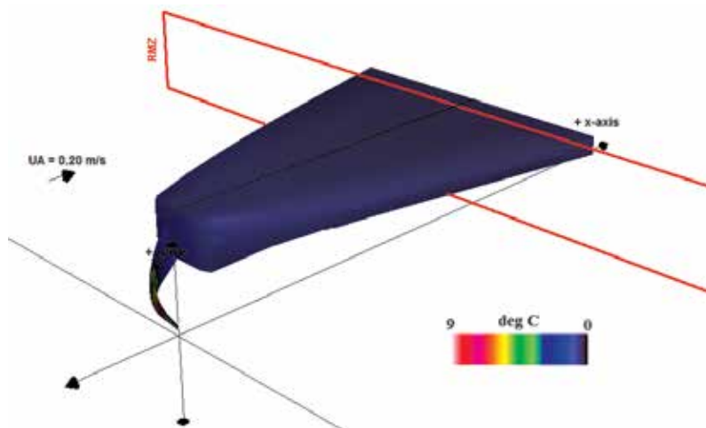
Fig. 2. Scenario I brine plume from the single port discharge
