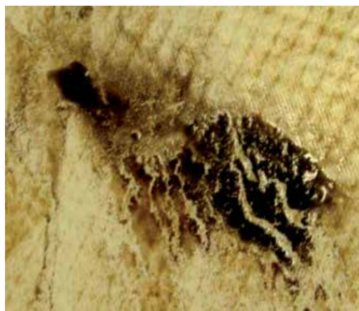
Fig. 10. Deposit of MnO_2 on RO membrane
