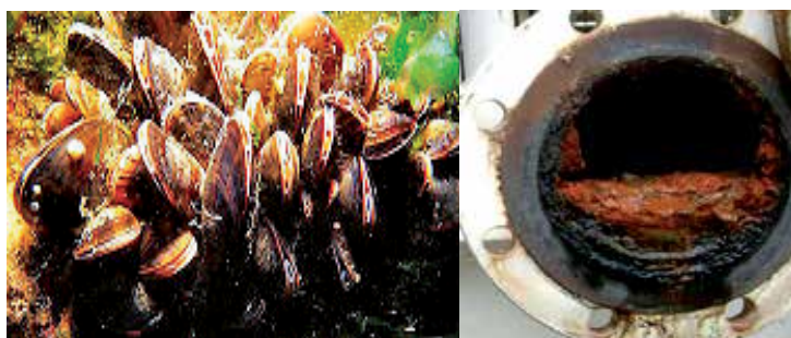
Fig. 21. Mussels development on intake (left) and biofilm on pipes (right)
