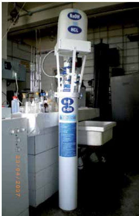
Fig. 8. Photography of a pilot one body multi stage multi cell water deionization filtration device
