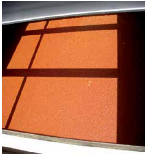
Fig. 31. Sludge blanket at the top of the flotator (Spidflow™)
