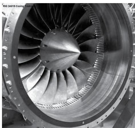
Fig. 12. EJ200 LPC with axial slots casing treatment (Broichhausen & Ziegler, 2005)
