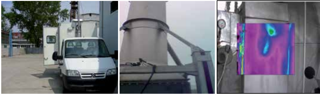
Fig. 13. Mobile laboratory at INCDT COMOTI (left), emissions measurements at the stack (centre) and sighting area of Fluke camera (Ti45FT type) with sound level meter (right)
