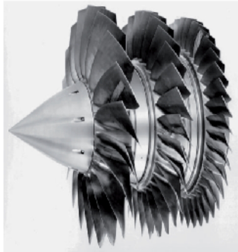
Fig. 7. Low pressure compressor of the Eurojet EJ200 turbofan engine fabricated with the BLISK technology.
