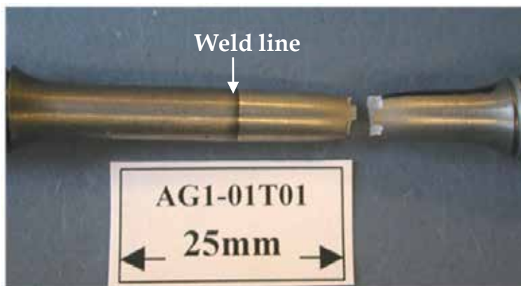
Fig. 19. Photograph of a tested tensile specimen. Note the fracture at the right side, far from the weld line.
