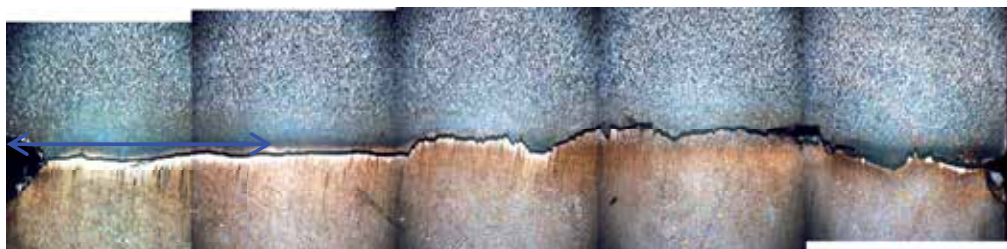
Fig. 23. Crack path for fracture toughness specimen corresponding to K_{Ic} = 15 MPa.m 1/2 .
