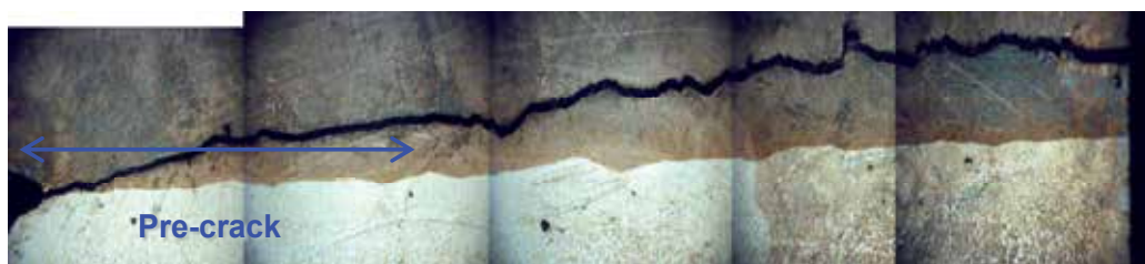
Fig. 24. Crack path for fracture toughness specimen corresponding to K_{Ic} = 45 MPa.m 1/2 .
