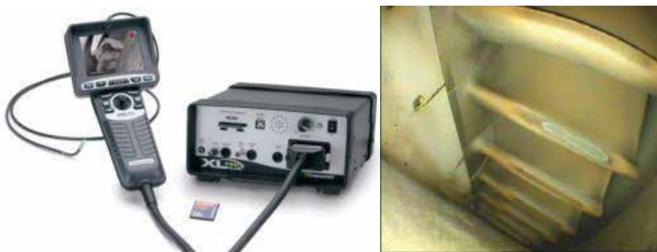
Fig. 13. An industrial videoscope and an image of gas turbine blades condition (Reports, 2000-2010)
