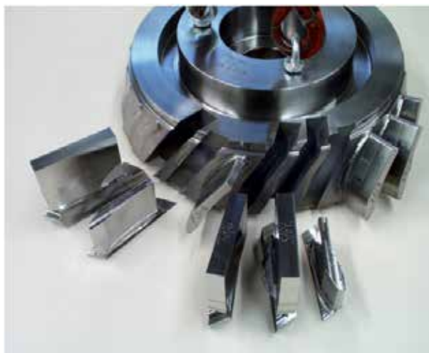
Fig. 26. Pre-machined BLISK demonstrator, after extraction of blade-blocks.
