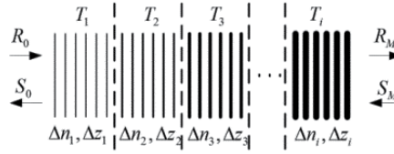
Figure 2. Transfer matrix method used to obtain the spectral characteristics of a fiber Bragg grating ( \Delta n - average index of refraction, \Delta z - section length, R_0, S_0, R_M, S_M - electromagnetic waves amplitudes)
