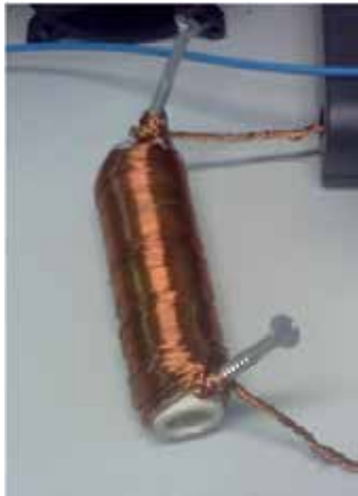
Figure 29. Assembled activation coil, designed according to the procedure described in [18]
