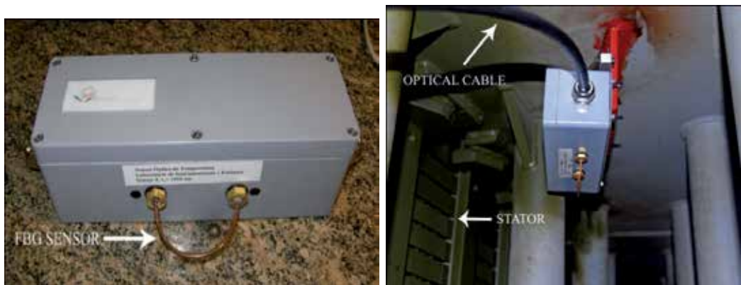
Figure 1. Box containing the optical fiber splices with the FBG inside the U-shape copper tubing (left) and installed inside the generator (right) (adapted from [2]).
