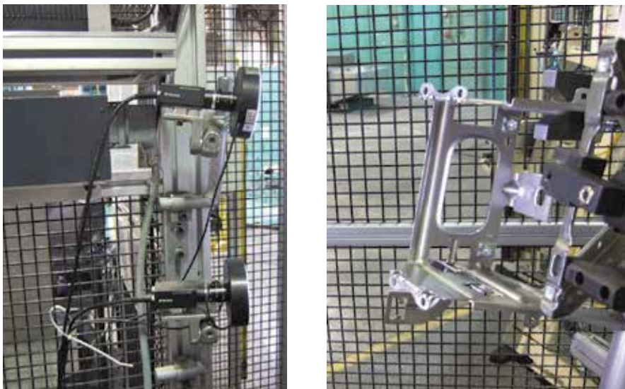
Fig. 4. Orientation of (a) cameras looking at bracket and (b) radio bracket in holder.
