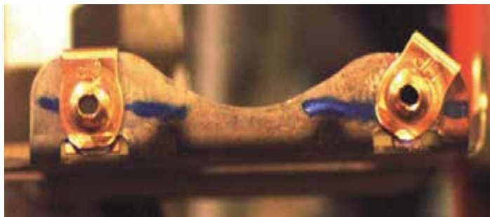
Fig. 9. Sample fail (backwards and upside down clip) for the orientation image set.
