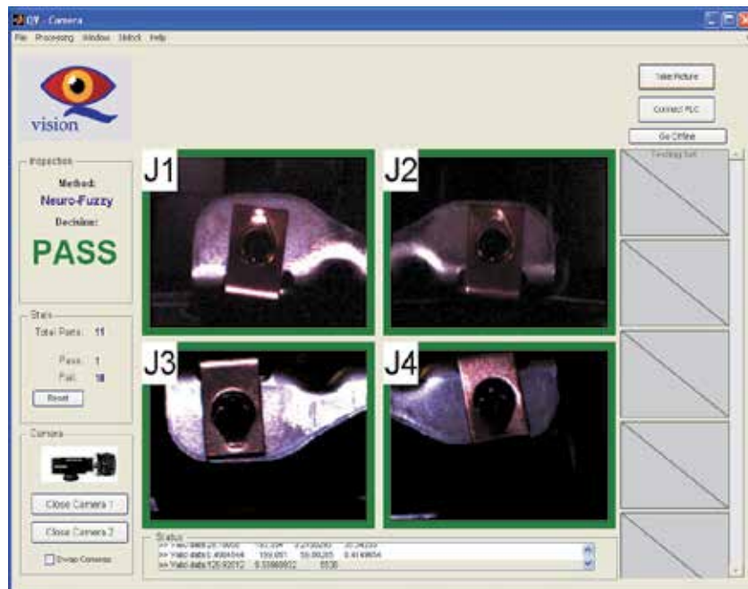
Fig. 5. QVision software GUI used to detect the presence of clips.
