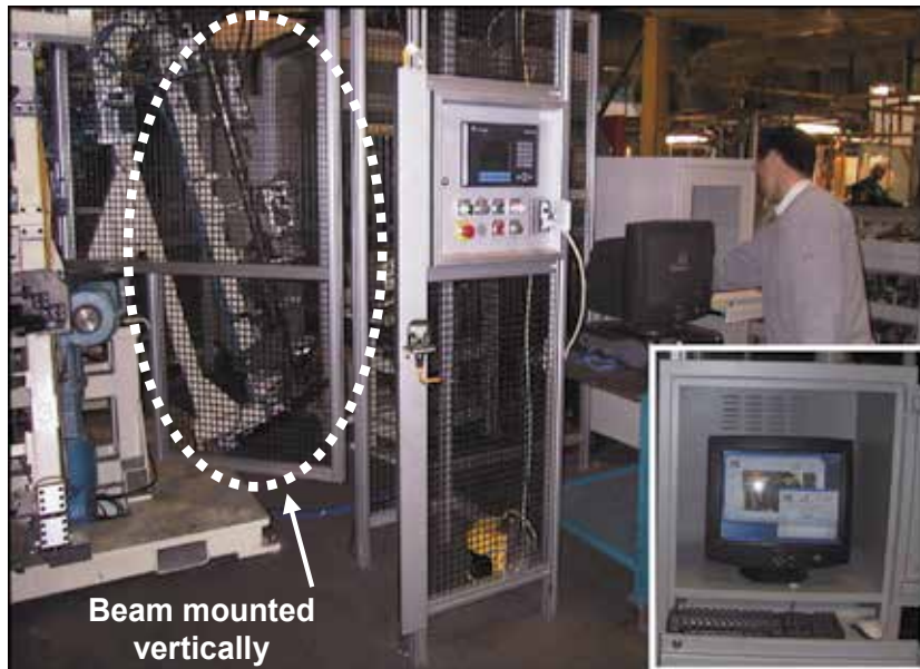
Fig. 3. PLC controlled manufacturing cell with PC controlled vision system.
