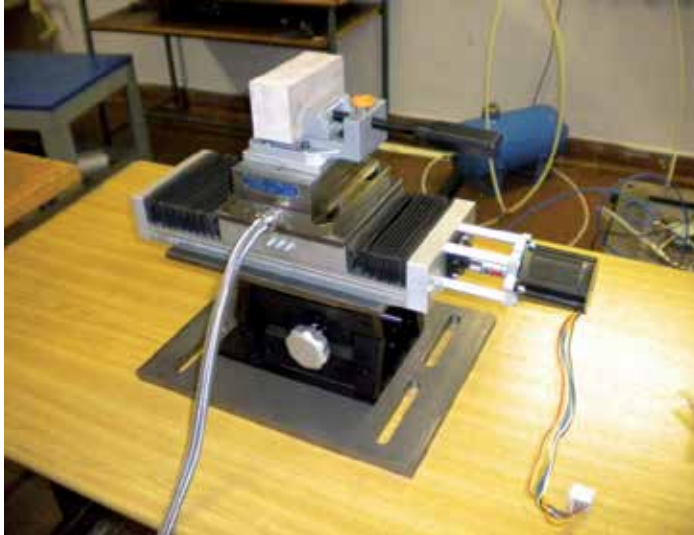
Figure 15. Motorized slide used for the dynamic tests
