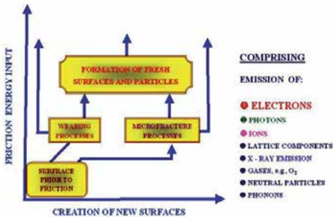
Figure 5. Physical processes evolved by friction.
