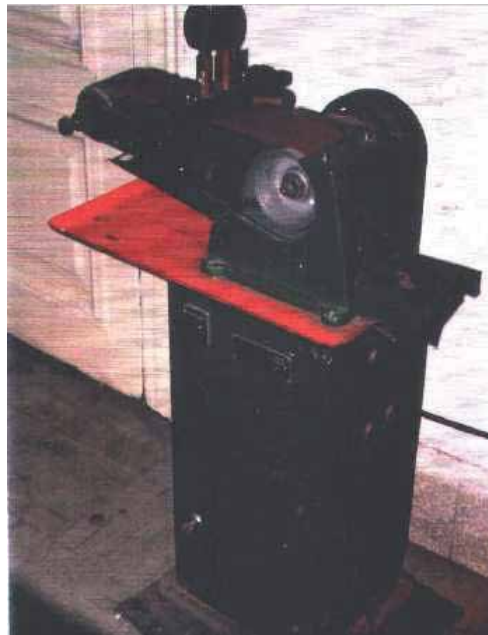
Figure 2. The pin-abrasion testing machine [19, 20]
