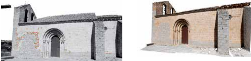
Fig. 11. Left: Back projection error on pixels with a magnification factor of 10. Right: Texture mapping as the result of the fusion of both sensors
