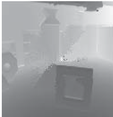
Fig. 11. The synthesized dense range map of the initial range values indicated in figure 10c.
