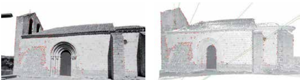
Fig. 10. Point matching based on epipolar constraints. Left: Digital image. Right: range image.
