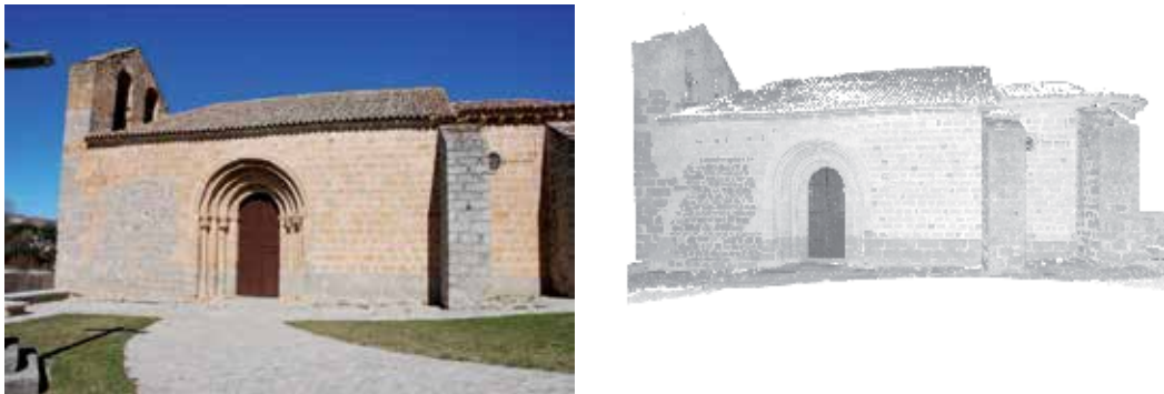
Fig. 9. Input data. Left: Image acquired with the digital camera. Right: Range image acquired with the laser scanner.
