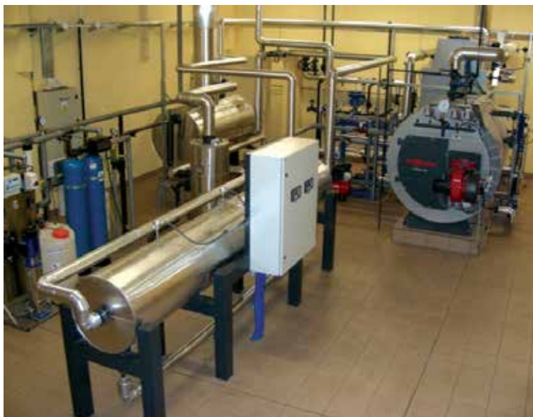
Fig. 11. View of the experimental installation for testing the computer system for on-line monitoring thick-wall pressure components
