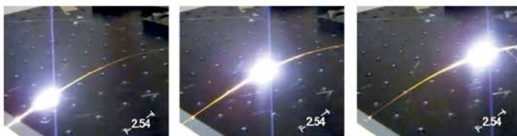
Fig. 3. Sequence of frames of the fibre fuse propagation in a SMF fibre, the time difference between pictures is 0.1s
