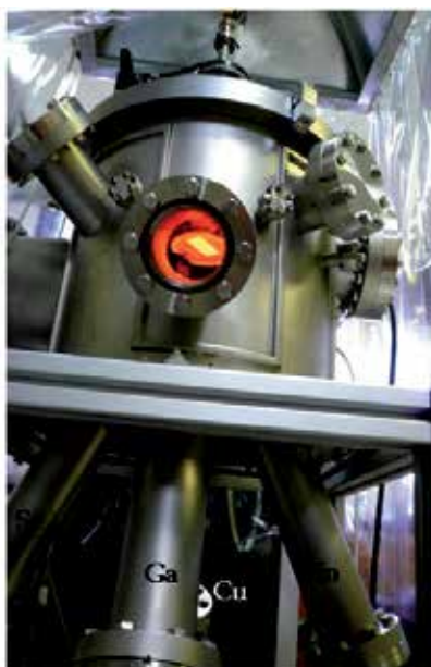
Fig. 8. Thermal co-evaporation system with Knudsen effusion cells to deposit Cu(In,Ga)Se 2 thin films
