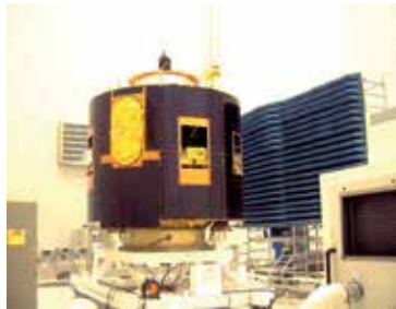
Fig. 17. Solar Array for spinning Satellite, Meteosat Second Generation (Credits: ESA - MSG Team)
