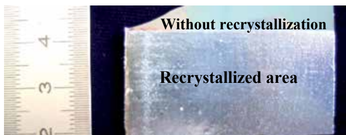
Fig. 3. Appearance of polycrystalline silicon absorber after recrystallization
