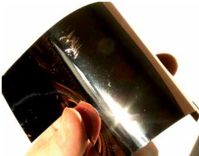
Fig. 14. Test structure of elastic CdTe layer based on UPILEX® foil and contacted by 2 μm Cu layer.
