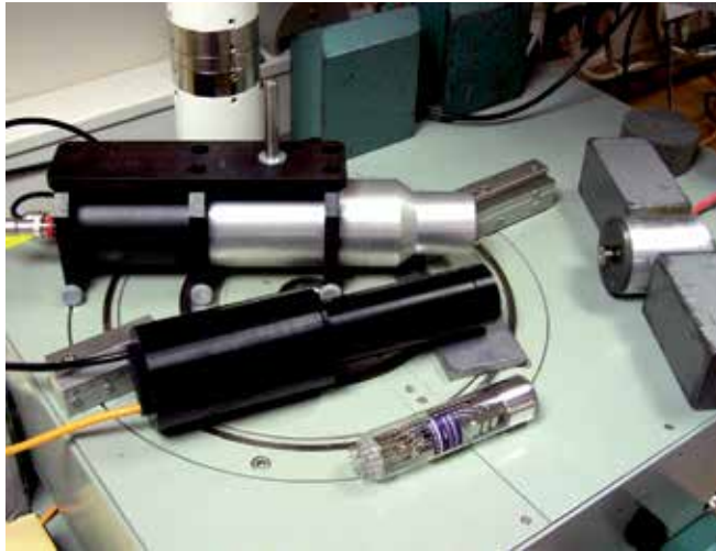
Fig. 6. High energy detector - upper, and low-energy detector - lower; and simply PMT.
