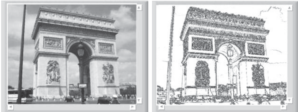
Fig. 12. Sobel Edge Detector. (a) Grayscale image, (b) Sobel Transformation.
