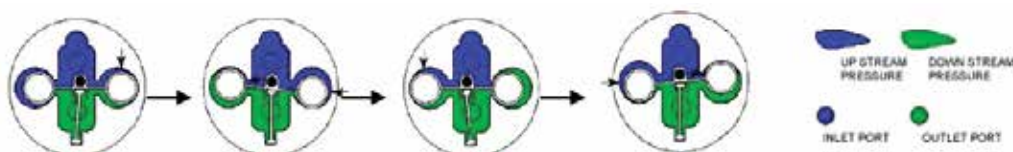
Fig. 8. Flow measurement principle for the flow meter. Pistons movement inside the chamber while the liquid passes through the flow meter (DEA, 2008)
