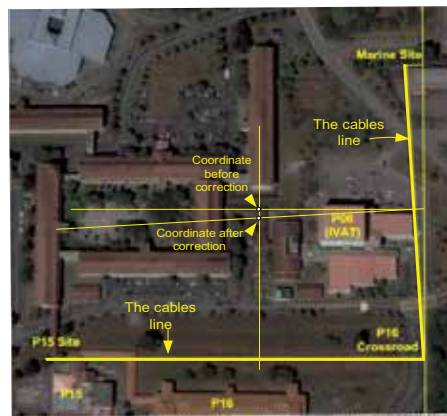
Fig. 10. Correction for the Y-axis of the 'imperfect' Cartesian system
