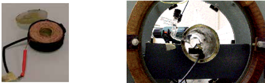
Fig. 5. The transmit-receive coil (left figure). On the right figure, the coil could be seen inside the Helmholtz coils and the shield. The coil is loaded by a sample consisting of Pyrex (a type of glass) cylinder filled with pure water.
