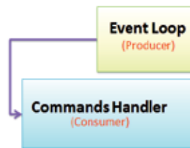
Fig. 16. Queued State Machine-Producer Consumer architecture used for the VI's programming
