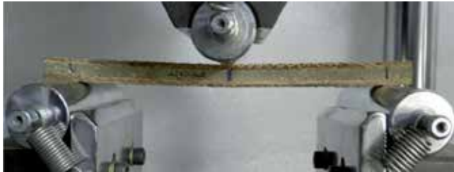
Figure 4. Sandwich sample mounted on flexural test set-up
