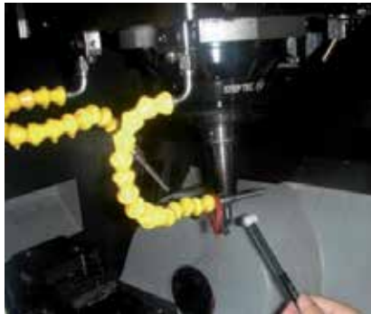
Figure 15. Experiment setup for modal shapes of spindle-tool system
