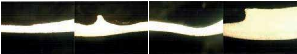
Figure 11. Macrograph of 5-7 o'clock position showing the absence of ERW.
