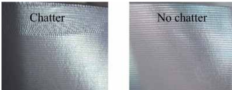
Figure 19. Comparison of finished blades using different spindle speeds, (L) from deterministic optimization (R) from robust optimization
