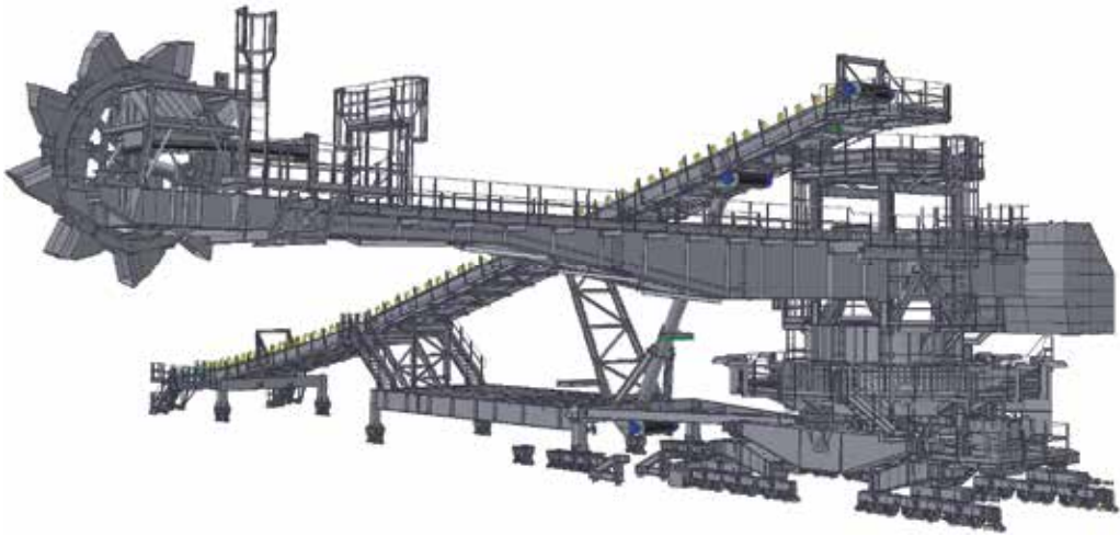
Figure 3. Stacker-reclaimer machine, overview – modeled by Inventor
