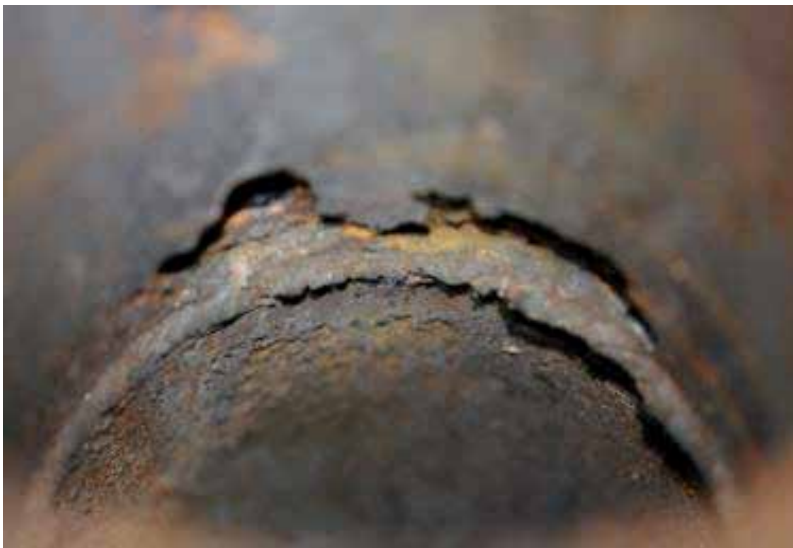
Figure 15. An excessive overfill and severe surface degradation beside overfill at 6 o'clock position.
