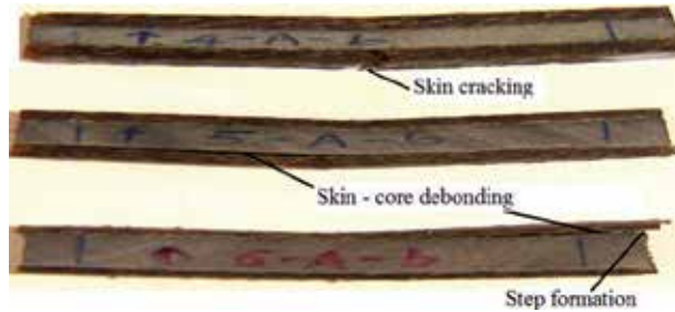
Figure 13. Sandwich failure modes under three point bending loads
