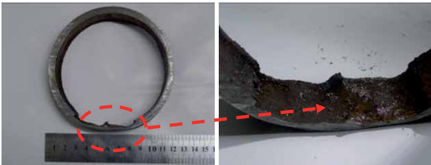
Figure 9. Uniform attack at the burst area from 5-7 o'clock position.
