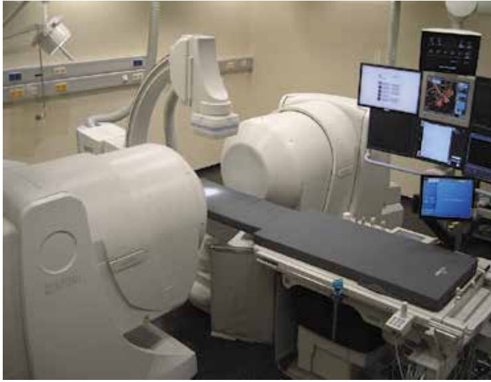
Fig. 3. Catheter suite with a magnetic navigation system (Niobe). Permanent magnets to both sides of the fluoroscopy table can be moved inside their casings to alter the magnetic field.
