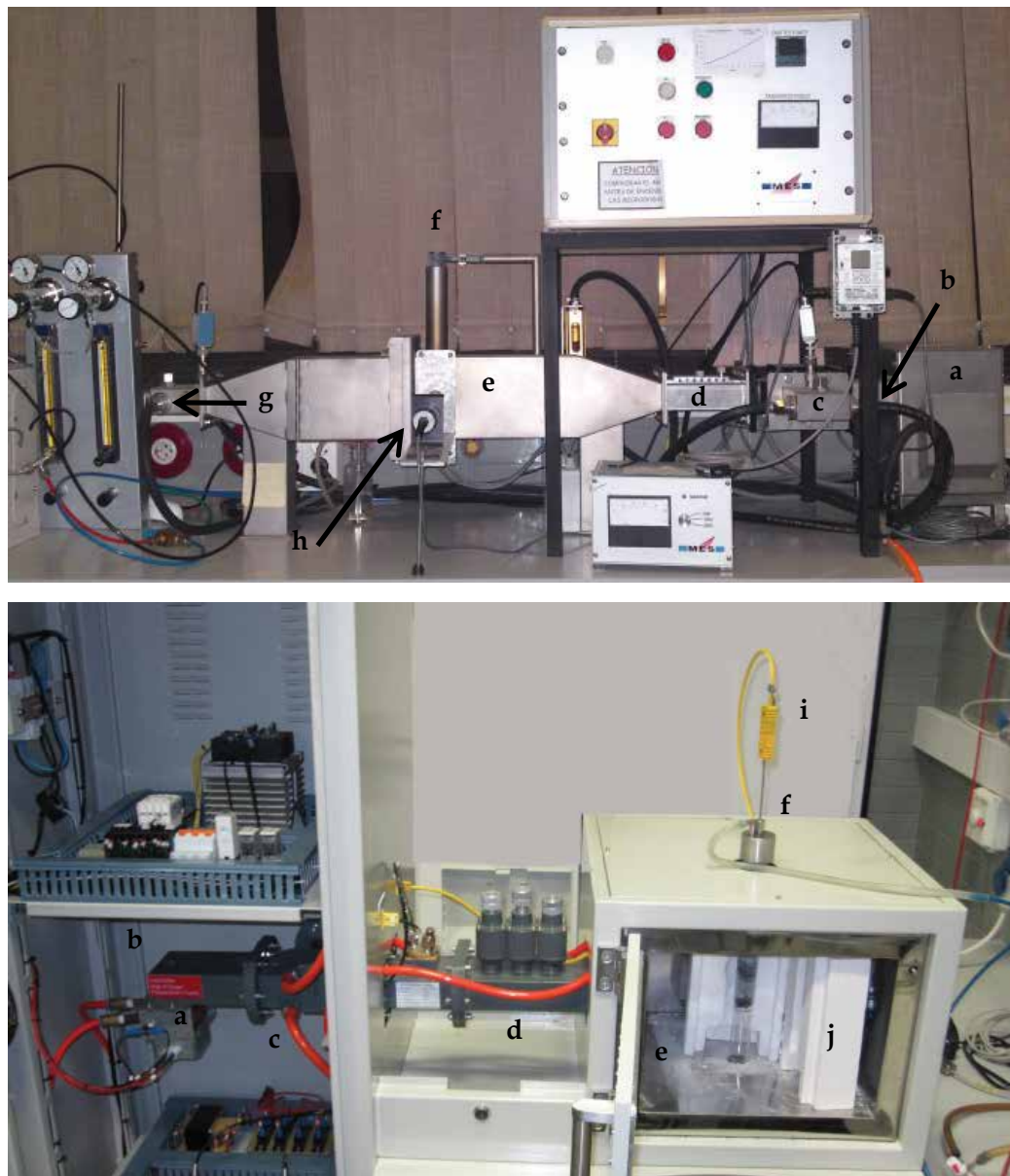
Fig. 1. Photographs of singlemode (upper) and multimode (lower) microwave ovens at INCAR ( www.incar.csic.es ) showing: a) magnetron; b) waveguide; c) circulator with reflected power meter; d) tuning screws; e) resonant cavity; f) reactor; g) terminator with transmitted power meter; h) infrared optical pyrometer; i) thermocouple; and j) insulating material
