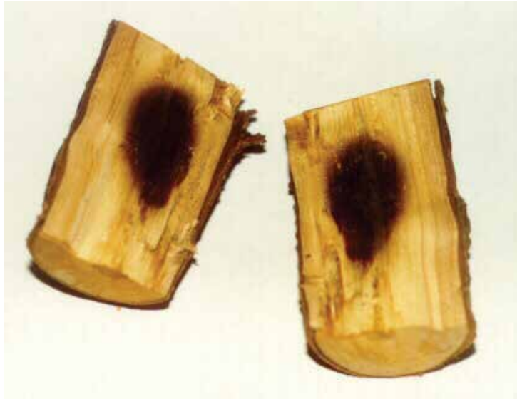
Fig. 11. Charring, due to thermal runaway, in the core of a wood sample that was being dried in a microwave oven (Note: the location of the charring in comparison with the last image in Fig. 7)
