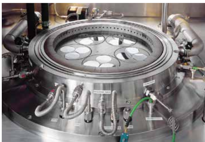
Fig. 2. Typical reactor arrangement for epitaxy processes
