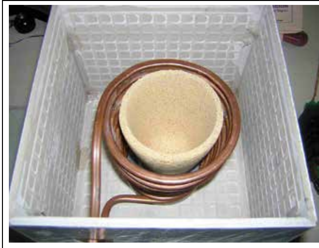
Fig. 9. Melting furnace partially assembled
