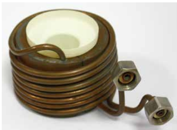
Fig. 8. Evaporator with inductor-concentrator equipped with crucible, which allows avoiding migration of liquid metal towards the outer crucible surface
