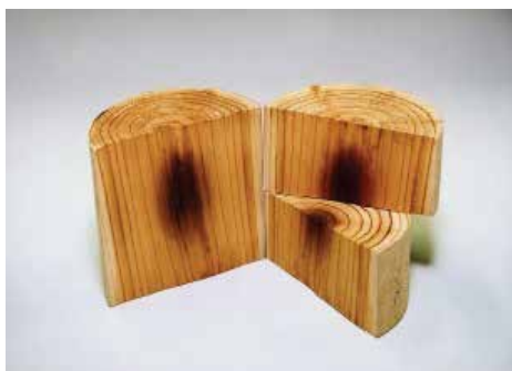
Fig. 5. Cross-section of wood after 3 minutes of microwave radiation (Reprinted from Miura et al., 2004, with permission from Elsevier)
