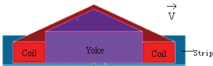
Fig. 1. New structure of the TFIH equipment
