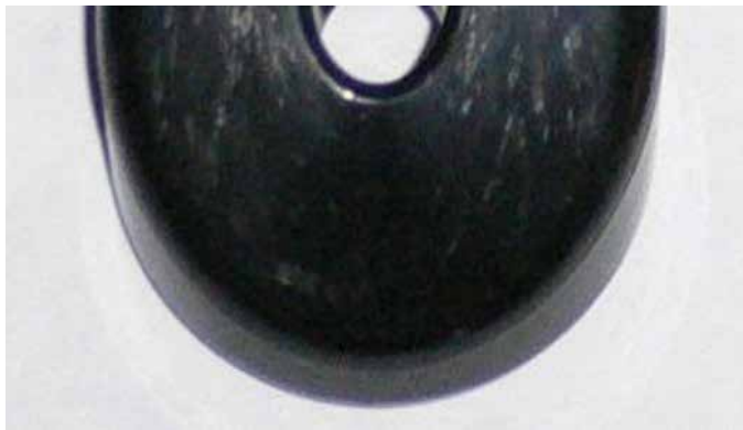
Fig. 3. Warpage and silver streaks at bottle Opener
