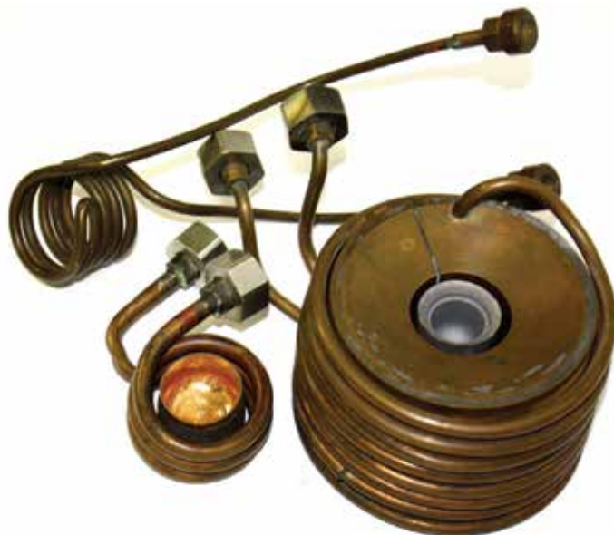
Fig. 2. Photographs of water-cooled evaporating inductors for use in electronics, two of them are shown with crucibles. The left inductor has the top turn with opposite winding as compared with the rest turns
