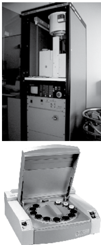
Fig. 1. Atomika Extra IIA TXRF Spectrometer and PANalytical MiniPal2 benchtop XRF Spectrometer
